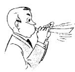
We can explain this easily. Because of your blowing there is an area of low pressure above the paper. Under the paper the air is not moving and so the pressure remains normal, Thus, the pressure under the paper is greater than it is above and, as a result, the paper is pushed upwards into a horizontal position.
