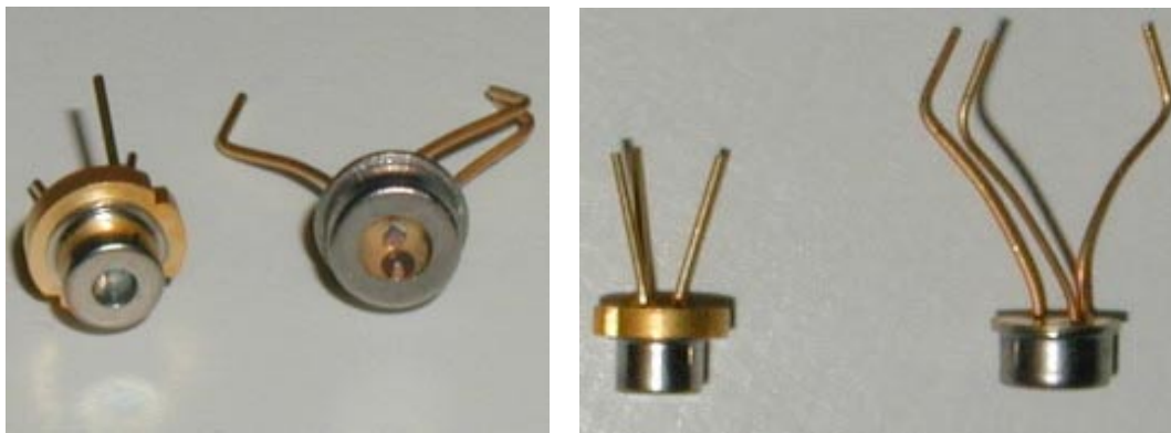
Figure 53: Lumex diode (on the left side of both pictures, golden rim) compared to the Honeywell VCSEL diode (on the right side of the pictures, longer legs)
