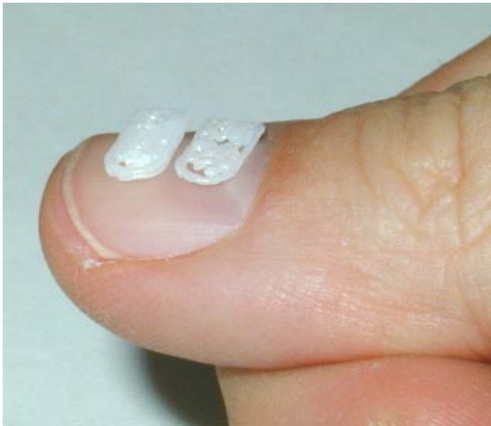
Figure 100: 3D printout of the two servo arms: on left the side the 1.0mm thick one, on the right side the 0.5mm thick one. This is definitively the limit of our current 3D printer, at least with the current print heads (T16). Basically, the piece consists of one layer of ABS traces, trying to fill the plane (not very successfully)
