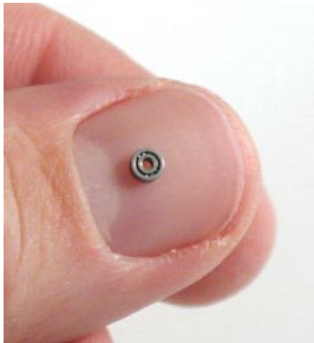
Figure 94: Miniature ball bearings with an outer diameter of 3mm, for the 0.9mm axle
