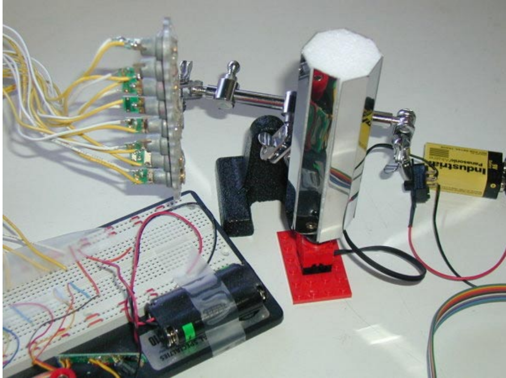
Figure 17: First prototype with 8-faced mirror with Lego motor.
