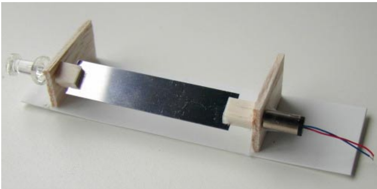
Figure 42: full rotation two-faced mirror balsa test assembly
