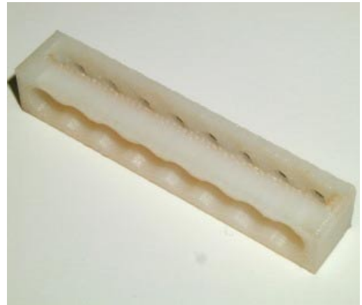
Figure 77: 3D printout of the clip and holder design. Did not work at all, since the legs of the clip were built up vertically, so they consisted of many slices of small size. In addition, the tips of the six legs were overhanging, so the 3D printer had to build up a considerable amount of support material around the legs, which is always problematic since the boundaries are not that precise.
