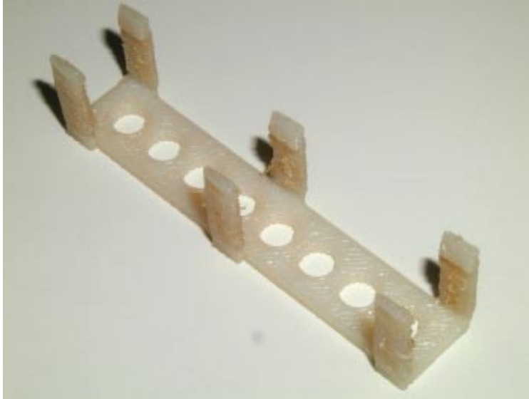
Figure 77: 3D printout of the clip and holder design. Did not work at all, since the legs of the clip were built up vertically, so they consisted of many slices of small size. In addition, the tips of the six legs were overhanging, so the 3D printer had to build up a considerable amount of support material around the legs, which is always problematic since the boundaries are not that precise.
