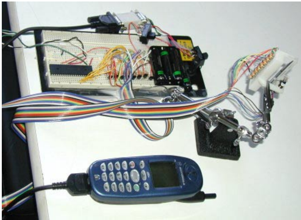
Figure 113: TinyProjector prototype 9 connected to a iDen cellphone via serial cable
