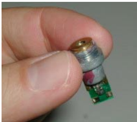
Figure 8: From these key chain laser pointers, the laser diodes are extracted.
