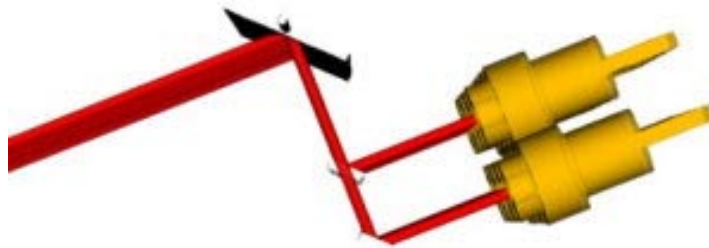
Figure 20: Design with two rows of 4 laser diodes
