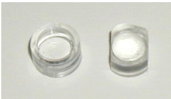
Figure 63: On the left side an original lens, as salvaged from a key chain laser pointer, diameter 7mm. On the right, a modified lens with sides sanded down to an overall width of 5mm.
