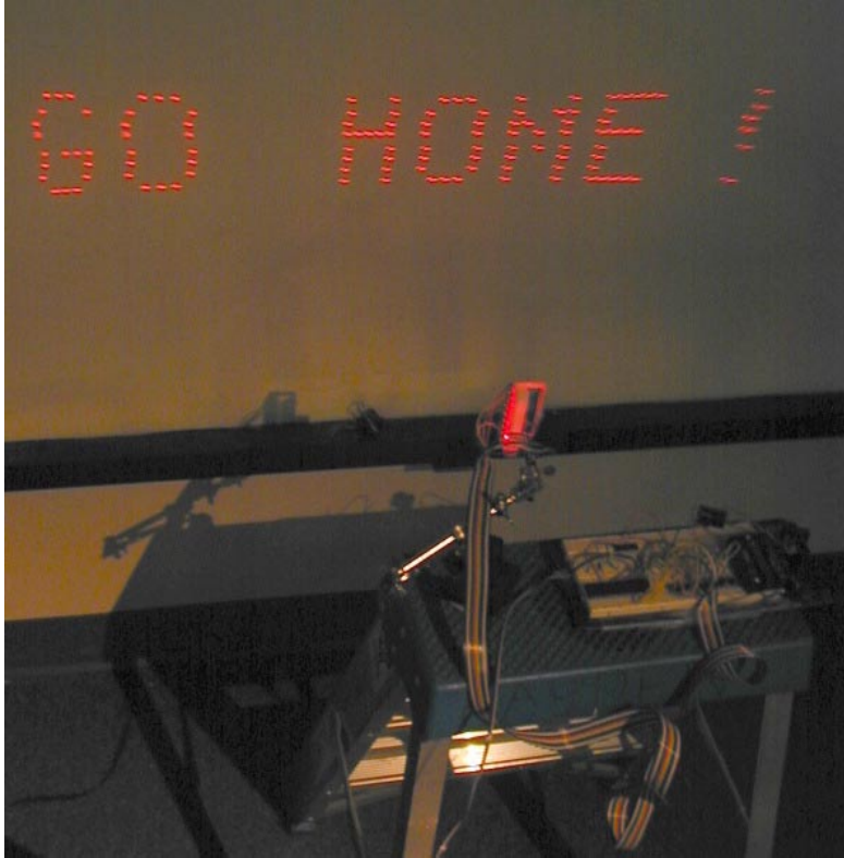
Figure 115: Example projections, and a close-up of TinyProjector prototype 9 in the dark (above).
