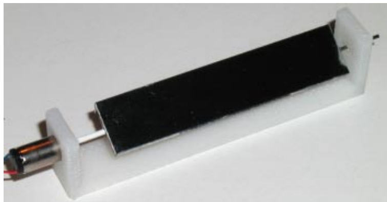
Figure 95: 3D printed U piece (prototype 6) with rotating mirror (axle 0.9mm, 6mm pager motor, direct drive)
