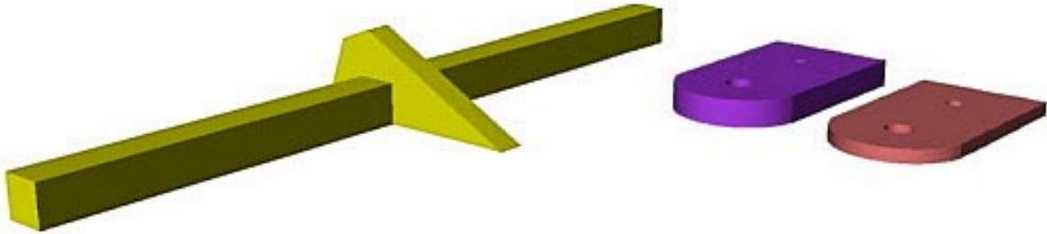
Figure 99: Design of the mirror holder and the servo arm. It looks nice in the modeling software!
