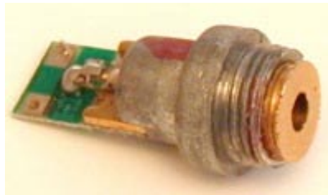
Figure 8: From these key chain laser pointers, the laser diodes are extracted.
