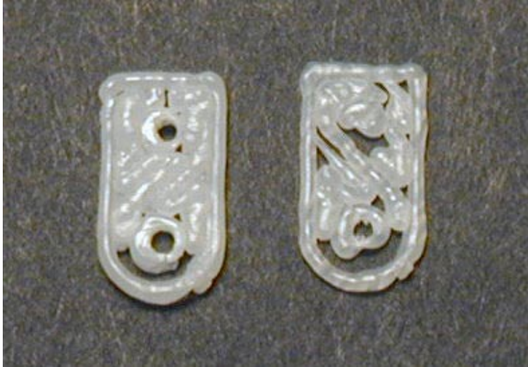
Figure 101: Close-up of the two 3D printed servo arms. The limitations of the printer are clearly visible
