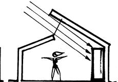
This thermal storage wall uses water-filled vertical tubes. To provide more control of heat flow into the house, a normal interior wall separates the water wall from the living space. A thermostatically-controlled fan circulates room air past the warm tubes. At night, an insulating thermal curtain is drawn across the glass. Corrugated, galvanized culverts and fiberglassreinforced polyester tubes are the more commonly used cylinders.
