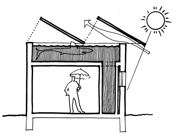
The "Cool Pool" concept is being developed and tested in Davis, Indio, and Sacramento, California, by Living Systems. The roof pond radiates its heat to the sky. The coolest water settles down into the radiant wall panel, cooling the house. The warmer water rises up into the pond where it radiates to the sky.
