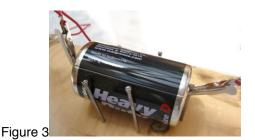
2. Stick a 2 in piece of foam tape on the bottom of each of the two batteries, and then remove the backing material. Place the batteries on the base in the approximate positions shown in Figures 1 and 6. NOTE: For a more robust permanent mounting of the batteries, use 6 nails for each battery to make a battery holder as shown in Figure 3. If you are going to use the nails, it is preferable to do the hammering at this point, rather than after other components are installed.
