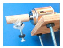
To operate Skippy, just stand it on its legs and connect the wires so that that the motor starts. The dowel with its eccentric attachment spins, the whole creature vibrates, and when you let go it will start "walking."
