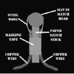
Figure 13-3: Diagram of an electric igniter.
