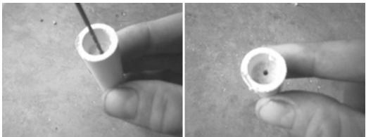
Figure 11-1: Drilling a 1/16-inch hole in the top clay cap down to the delay mix.
