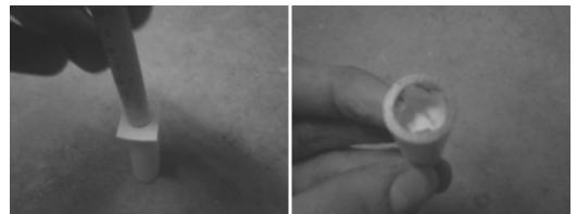
Figure 11-3: Press a small piece of paper into the top of the motor to hold the black powder in place.
