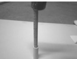
*Figure* 8-8: *Ramming the propellant into the bottom of the tube with a ramming tool and hammer.*
