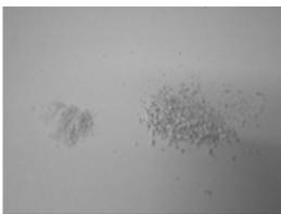
Figure 4-3: Left – cat litter after milling with a coffee grinder. Right – course cat litter out of the bag.
