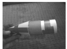
Figure 16-15: Nose cone glued on nose cone assembly.
