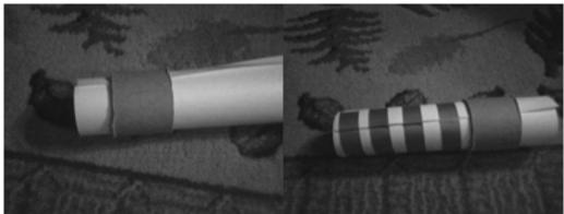
Figure 16-10: Rolling and taping cardstock to make a tube insert for the nose assembly.
