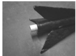
Figure 12-2: Motor inserted into model rocket with thrust ring sticking out.
