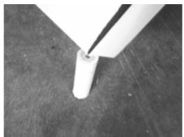
Figure 12-3: Filling the core with black powder.
