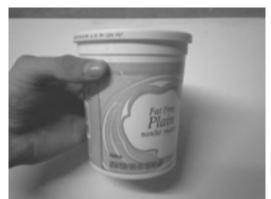
Figure 7-7: Shake the propellant in a plastic container with a lid to mix it.
