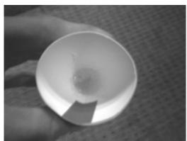
Figure 16-14: Fill the nose cone with hot glue to make it hard.
