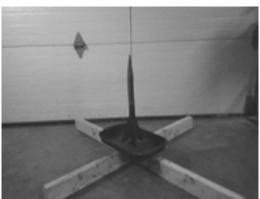
Figure 17-4: A finished launch stand with a rocket loaded on and ready to go.
