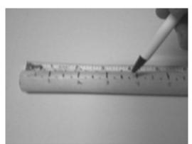
Figure 5-1: A dowel ramming tool with <sup>1</sup>/<sub>4</sub> inches marked off.
