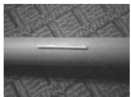
Figure 16-23: A drinking straw is used as a launch lug on the side of the rocket.
