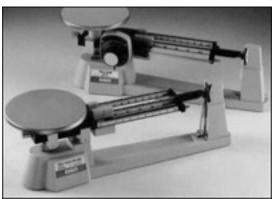
Figure 7-4: Scientific triple beam balance.
