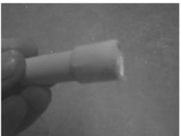
Figure 12-1: Masking tape "thrust ring".
