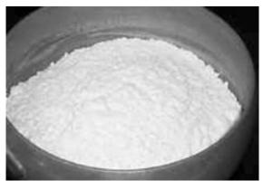
*Figure 7-8: The propellant should look like the powdered sugar and should be a fine white powder.*
