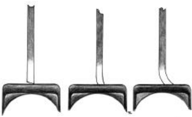
A bar end that is out-of-square causes bending
