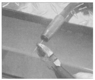
5.10 It's important to keep a pair of side-cutter pliers handy at all times to your MIG welder. Not only do you need it to maintain the correct protrusion of the wire from the nozzle, but when the wire develops a ball on the end, the arc is easier to start if you snip the ball off.
