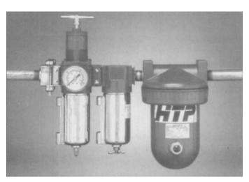
7.30 The Max-Dry from HTP is a three-stage system. Stage one is a self-draining 5-micron filter, stage two is a "coalescing" filter, and the final stage is another filter with a large amount of desiccant. The desiccant changes color when it can't absorb any more humidity, but can be dried out in an oven for reuse.
