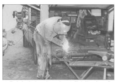
1.3 The farrier of today works out of a truck, filled with equipment like a grinder, drill press and welder, all running on AC power when available; otherwise, horseshoes are shaped in a portable forge. Today's blacksmith has the advantage of tools like this MIG welder that speed up making special horseshoes.
