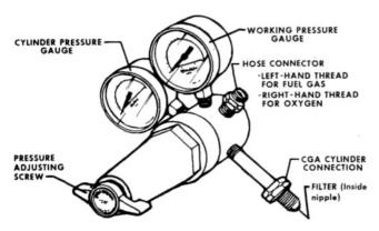
3.10 The gauge/regulator setup screws onto the tank's cylinder valve, and has a fitting for attaching the hose leading to the torch.
