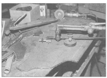
3.56 The same tool can be used, with different attachments, to cut a perfect circle of any size from a few inches to two feet in diameter. Removing as much of the human element of hand control makes for better parts that require less grinding to finish.
