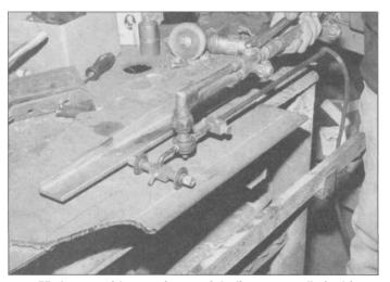
3.55 A great aid to cutting straight lines manually is this "compass" guide. It holds the torch tip firmly, but in a swivel arrangement that allows it to turn as you move along the line, and the torch stays the same distance from the work and much steadier. Here it is being demonstrated against another great tool, a magnetic steel guide that sticks strongly to the work and saves the hassles of setting up a bar or tube with some clamps.
