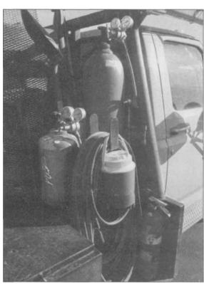
3.12 In industrial situations, like this oilfield service truck, gas welding setups may be equipped with large cylinders and 100 feet of hose, to handle any situation.
