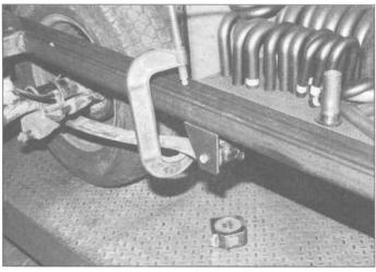
9.22 The front spring-mounting plates are bolted onto either side of the front spring eye, squared to the rails and clamped lightly in position for tacking.
