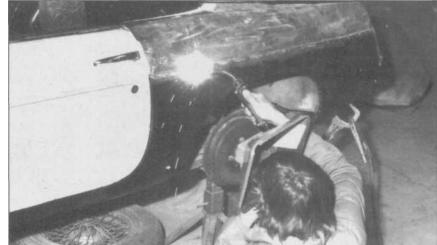
5.1 The use of wire-feed MIG welding has expanded greatly in the last ten years to encompass body shops, muffler shops, race-car builders and home hobbyists as well as the industrial production work it was designed for. It has advantages of speed, simplicity, cleanliness, and the ability to work well on thick and thin materials.
