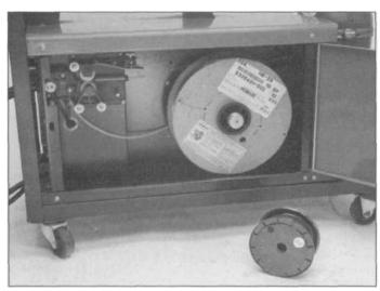
5.34 Inside the wire-drive portion of a typical small MIG machine, this machine comes with a small wire roll such as at lower right, but comes with an adapter to handle the larger rolls such as in the machine. The small wire rolls are inconvenient unless you do only small projects.
