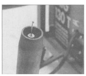
5.8 The wire must fit the contact tube closely, as this is where power is transmitted to the electrode wire. Note that the contact tube is recessed inside the nozzle, and the wire sticks out 1/2-3/4-inch from the nozzle.
