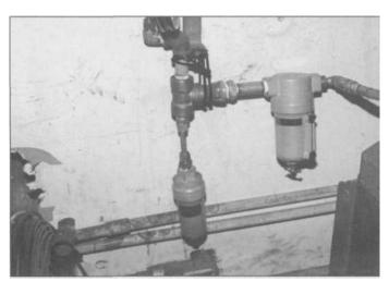
7.29 You can't have the air too dry for use with a plasma cutter. If your compressor is outside or a long distance away, use an extra filter/drier on the wall where the hard line switches to the flexible hose for your plasma cutter.
