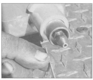
8.34 Small-headed copper-plated "studs" are inserted into the magnetic head of the stud setter.
