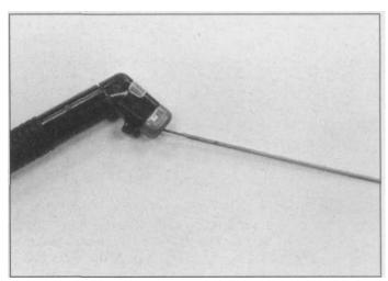
4.18 To achieve a different rod angle with a short-stub electrode-holder, just bend the rod near the holder to the desired angle. In some situation, where you have to reach down inside something to weld, the rod can be bent straight out.
