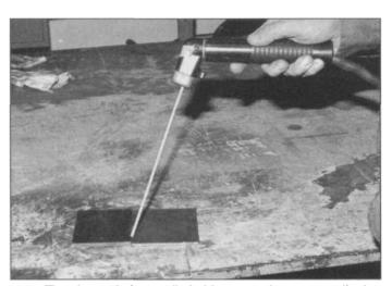
4.16 The electrode is usually held more or less perpendicular to the welding surface to start the arc, then laid back to continue the bead. Some weldors prefer a forehand technique, others a backhand direction, such as here.
