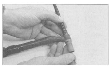
6.29 The sharpened tungsten is inserted into the torch body, and when the tip is sticking out the right distance, you tighten the back cap to hold it in place.
