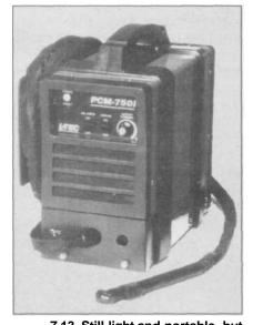
7.13 Still light and portable, but powerful enough to cut 3/4-inch steel, The L-TEC PCM-750i has 50 amps with a 40% duty-cycle at that setting, and has its own torch storage spool and spare parts storage compartment.
