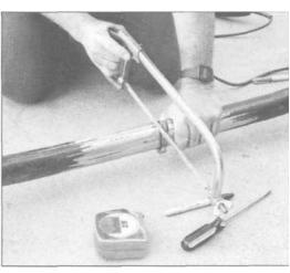
9.7 Grind the paint from the center of the axle, mark a straight centerline across the axle for lining-up purposes later on and cut the axle with a hacksaw. A hose clamp around the axle is used as a saw guide to keep the cut straight.
