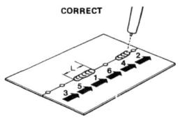
5.51 When working on large panels of thin material, such as when doing body work like welding on a new quarter-panel, warpage is a problem unless you keep the heat down by making lots of tack welds, then switching back and forth to the coolest section to add a short weld, then move to another section, and switch back and forth until the whole seam is done. A continuous weld might put too much heat in, and warp the new panel, requiring lots of hammer-work to straighten.
