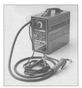
5.16 A popular entry-level MIG machine is this 110-V Pocket-MIG from Daytona MIG. Though it weighs only 42 pounds, it has an amp range from 30-110 amps, capable of welding up to 1/4-inch steel. Very portable, it's ideal for home/shop use, especially on sheet metal.
