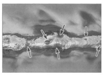
3.37 There is some silicon slag after brazing (arrows), which can be softened with water after the part cools enough so that water will not warp it, then the rest comes clean with wire-brushing.
