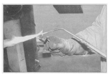
3.22 To start a torch, open the acetylene valve 1/2 turn and light immediately with a striker like this. Never use a match, cigarette or lighter, you could easily burn your hand. Once the sooty acetylene is lit, gradually add oxygen until you achieve a neutral flame.
