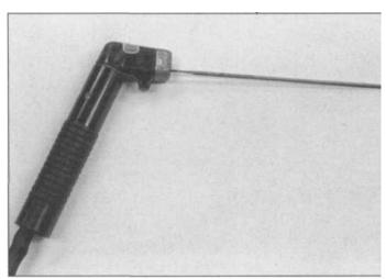
4.17 Arc-welding electrode holders are usually a clamp-like affair, with notches to allow the rod to be clamped at several different angles. Many arc weldors prefer this style, called a short-stub, in which the rod is inserted and the handle is twisted to lock the rod in place.
