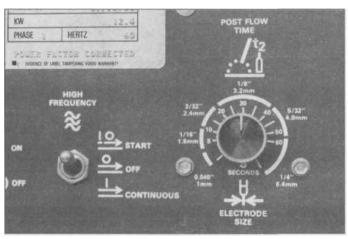
6.22 The three-position switch at left is for the highfrequency, and at right is the post-flow timing as related to various sizes of tungstens. The bigger the tungsten, the more post-flow timing to cool it off.
