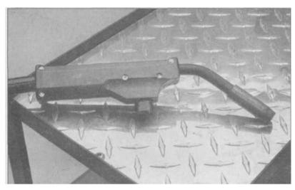
5.7 The basic MIG torch is quite simple. Inside is a guide tube that the wire comes through, a switch that turns on the power and the shieldinggas flow. The curved neck, called a "swan neck", holds the contact tube and the nozzle.
