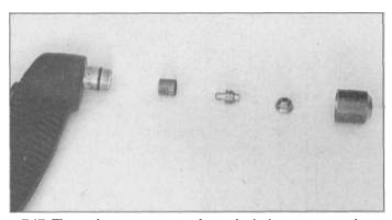
7.17 The main components of a typical plasma-arc cutting torch are, from left: torch body with o-ringed and threaded extension, the swirl ring, the electrode, the cutting nozzle, and the retaining cup. Some brands have a slightly different arrangement of parts inside.
