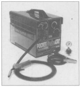
5.17 A 110-V, 130-amp MIG is made by several companies for the home/shop market, this one is by Daytona MIG and welds up to 5/16-inch steel. It features a cooling fan and a 30% duty-cycle at maximum amperage, 95% at 30 amps.
