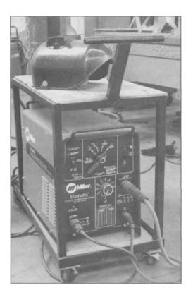
6.14 Less expensive, air-cooledtorch TIG machines have been available now for some time and are making inroads into shops where TIG was previously considered too expensive. This Miller "Econo-TIG" is being used in a street-rod shop on a homebuilt cart to make it as portable as any MIG machine.
