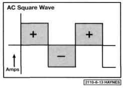
6.13 As a standard "sinusoidal" wave of AC current flows, it is constantly reversing its polarity and its output is always fluctuating as the wave flows. With the new square-wave technology, electrodes can be used at higher currents and have good arc staring and stability, but without the radio interference of traditional high-frequency superimposition. The square-wave design inverts the current much faster, for better welds on non-ferrous materials.
