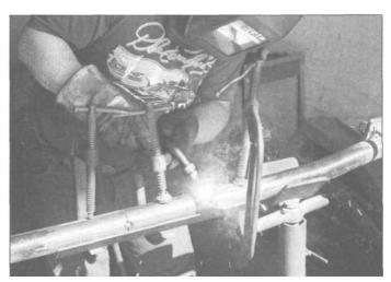
9.10 Here the assembly is tack-welded at several points around each joint with a MIG welder.
