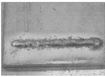
4.14 At right on this bead, you can see the dark gray slag coating covering the weld. The portion at the left has been chipped off to reveal a bright, shiny weld.
