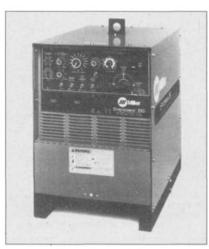
6.7 Most shop-type TIG welders are heavy, bulky power sources that require three-phase input power and water connections, making them less portable than other welding machines. This is a Miller Synchrowave 250, a popular unit in many fabrication and race-car shops.
