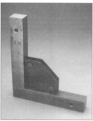
8.44 HTP and other companies offer these strong magnetic holders that can secure two pieces of tubing for angles of 45 degrees, 90 degrees, and 135 degrees. Tack the parts then move the magnets to the next joint.
