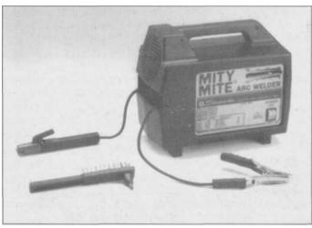
4.30 The Eastwood Company markets a lot of equipment and supplies for auto restoration, and this is their small 110V arc welder. At its maximum of 70 amps, it delivers a 10% duty-cycle, so you won't be welding any bridges together, but it only weighs 26 pounds, so it's extremely portable and welds up to 3/16-inch.
