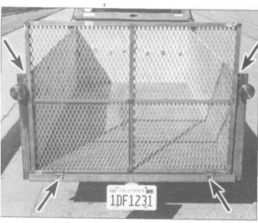
9.36 Our metal tailgate will save fuel because air flows through it on the road, cutting wind resistance. The frame was made of 1x1-inch tubing, to which was added steel mesh. Hinges (bottom arrows) were welded to the tailgate and bolted to the trailer. Top arrows indicate where tabs were welded to the gate for bolting with wingnuts to the trailer structure.
