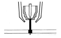
7.3 In the needle-arc version of plasma welding, the narrow-and-tall arc forms a weld that makes 100% penetration, top and bottom. The technique is used mostly in precision industrial applications.
