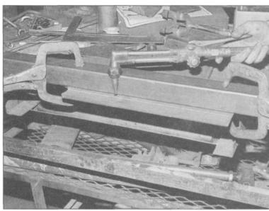
3.45 Clamp a piece of metal to your work that spaces the cutting torch head just the right distance to make your cut-line. The steadier your torch is held, the cleaner the cut. Travel at a very steady speed.
