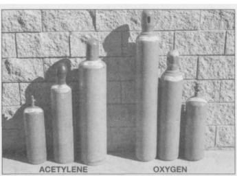
3.18 The small, medium and large welding cylinders contain 80,150 and 275 cubic feet of gas, but some manufacturers label theirs by a letter designation. Ask your welding supply shop approximately how long each size would last in terms of welding, and choose according to your needs.
