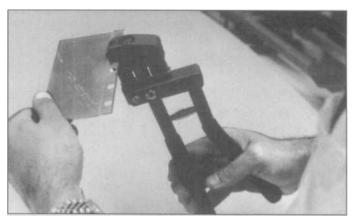
8.31 When you want to spot-weld sheet-metal panels that didn't have them originally, like new parts or repair panels you have made, a manual flange punch like this is a real help.
