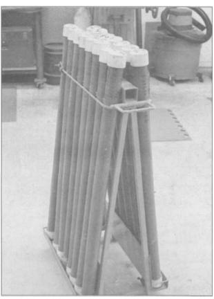
8.21 Weldor Bill Maguire made up this electrode rack for his TIG machine from a rolling platform holding 15 plastic plumbing pipes with caps, each marked for the size and type of electrode. A bungee cord holds them in the rack. Tubes keep the rods clean and dry.
