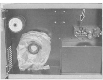
5.35 This is the drive section of a Daytona MIG wire-feed, which has a place inside to store an extra small roll of wire, good for keeping the spare clean if you occasionally switch to another type of wire for specific needs. Arrow indicates the knob for adjusting the wire roller tension.
