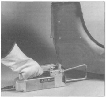
4.32 The spot welder is a self-contained mini-arc-welder, designed for joining sheet-metal panels on auto body work.
