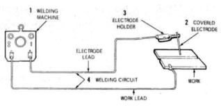
4.4 The layout of the arc-welding setup is simplicity itself. The rod (also called a stick, stinger or electrode) is both the source of the arc and the shielding gas, produced as the rod melts its flux coating.
