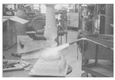
6.35 The rosebud tip on an oxy-acetylene torch is the easiest method for preheating thick and cast aluminum before heli-arc welding. In order not to warp cast-aluminum heads, manifolds and blocks, use heat-markers on the metal while preheating.
