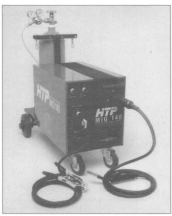
5.21 At the upper end of the 110V **MIG** scale are 140-amp units like this one from **HTP** America. It weighs 135 pounds, welds up to 1/4-inch steel, and has timing features such as stitch-welding and spot-welding.
