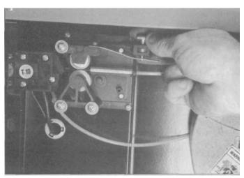
5.38 The wire tension is adjusted with a knob, and proper tension avoids wire-twisting problems inside the gun. The wire should be able to slip when it needs to. Most machines have a feature that allows you to retain the tension setting, once set, by swinging the tension arm away when changing wires.
