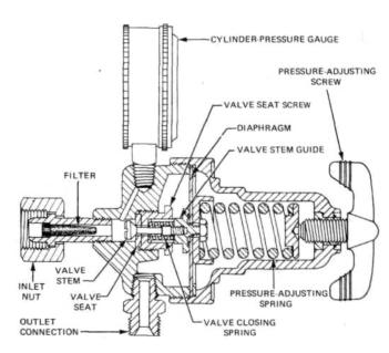
3.9 Cutaway of a single-stage regulator shows how the cylinder pressure is adjusted down to a usable range for welding. There are two gauges attached, one shows the total pressure left in the cylinder, and one shows the adjusted pressure supplying the torch.
