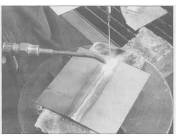
3.28 Before you are done, you will notice some movement or warping of the sample plates. If you plan to do automotive body work with a torch, you'll have to practice a lot on thin metal to get the hang of welding without burning holes or warping the work. Gas welding is not suited to the thin, high-strength body steels used on today's unibody cars.
