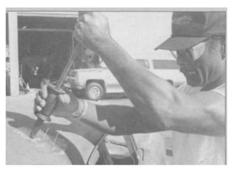
8.36 The suds are spot-welded in place, and a special slide hammer is used to pull out the dent or crease. Studs hold 500 pounds of pull.
