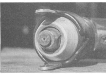
7.16 Eventually, enough material will blow back from cutting to cause a building of slag on the exposed nozzle and orifice of the torch, requiring periodic maintenance.
