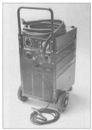
7.12 The bigger-amperage machines are all in the 220V category, and many, like this Daytona MIG Plasma Prof 50, require shop-type three-phase current, too. This one has a 35% duty-cycle at its rated max of 50 amps and 100% at 30 amps.
