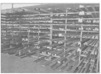
2.31 This steel supply store has a neatly-organized rack for materials, in which each different thickness of material is identified by a different color of paint on the ends, which makes shopping a lot easier for hobbyists without a micrometer.
