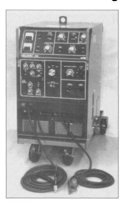
helpful on steel, but is essential on aluminum, magnesium and brittle, highstrength steels like the 4130 used in aircraft and race-car construction. It's called post-flow because it is post-welding gas flow. The post-flow of water and gas to the TIG torch also helps to cool the tungsten electrode down to the point where it can't oxidize when regular shop air flows around it after the welding stops.
