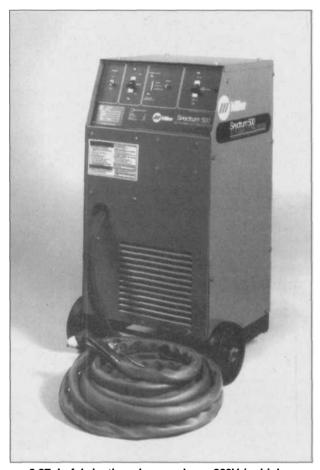
2.27 In fabricating shops, a large 220V (or higher current, three-phase) plasma cutter is used, capable of cutting thick materials and traveling at fast cutting speeds. Most plasma cutters are used without shielding gas, using air from the shop air compressor to cool the torch and form the ionized gas column under the tip that creates the arc.
