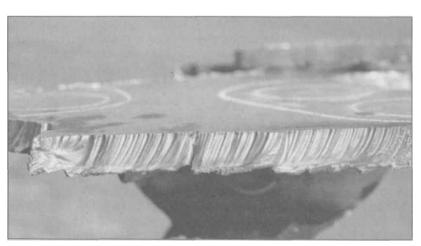
3.44 Examine the cut edge of plates after you have used your cutting torch. The proper heat and travel speed is when there is the least amount of slag along the bottom of the cut. This hand-held cut was moved a little too fast, as evidenced by the angled cut lines.
