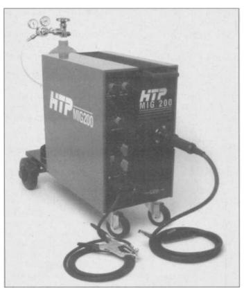
5.24 For welding up to 3/8-inch steel, a **MIG** like HTP's **MIG** 200 will do the job. It has 24 heat settings, up to 200 amps, and is suitable for farm or ranch work, commercial fabrication, or repeated automotive projects like building trailers or engine stands.
