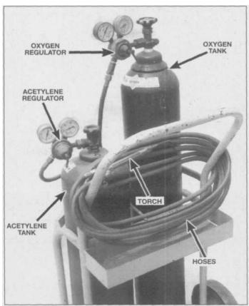
3.3 Look in the corner of almost any automotive or fabricating shop and you'll a setup just like this, with bottles, regulators, hoses and torch neatly corralled in a portable welding cart. Carts can be readily purchased, but most beginners like to make their own cart as their first project.
