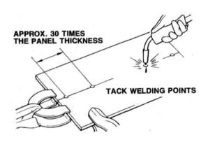
5.50 The thickness of the panel you are working on determines how far apart your initial tack-welds should be to firmly align your parts. On thin materials, you need a lot more tacks.
