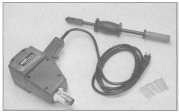
8.33 The HTP stud setter is a great boon to bodymen, who used to have to pull out creases and dents by drilling holes and using slidehammers that distorted the metal even further.
