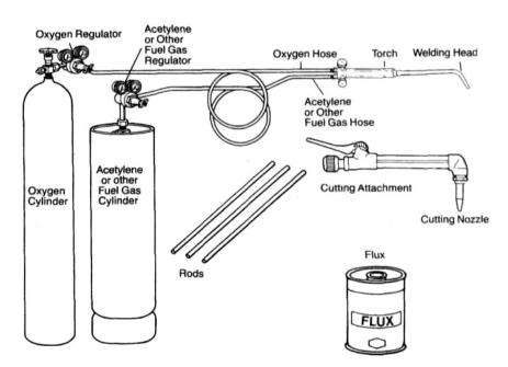
2.9 Gas welding with oxygen and acetylene gasses is one of the oldest forms of welding, and is still used today in construction, muffler shops and farm repairs. Its versatility lies in the ability to cut and weld, on thick and thin materials, and to do braze-welding as well. The flux shown is only used for brazing. Note the different size and shape of the two gas cylinders.
