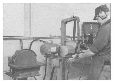
8.25 Ideally, you would have both a disc sander and belt sander for a variety of metal finishing needs. There are combination units, but beware of weak-powered sanders. When you put the rough edge of a 3/8-inch plate up there to sand, they stall easily.
