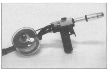
5.57 When MIG-welding aluminum, especially thin aluminum, the aluminum wire itself is fairly flexible, which can cause feeding problems inside the machine, because the drive rollers are *pushing* the soft wire a long distance. This is a spool gun, which holds a small roll of aluminum wire right at the gun for easy feeding.
