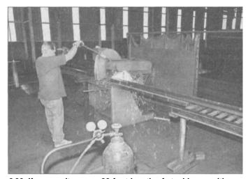
2.30 If you can't carry a 20-foot length of steel home with you, steel houses will generally make one "courtesy" cut for a small fee. Any cuts after that are expensive, so it's best if you have some method at home for cutting the metal for your projects.
