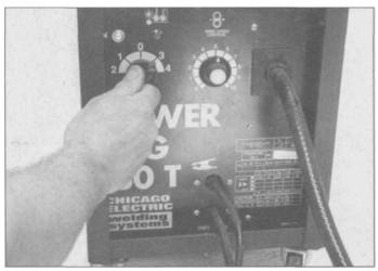
5.40 The basic MIG units have only a few power settings. Your instruction sheet will tell you the recommended thickness of metal for each setting, and a chart on the front of the machine usually tells you the amperage and duty-cycle of the settings. After some practice on different materials, you will learn instinctively which settings work best for your work.
