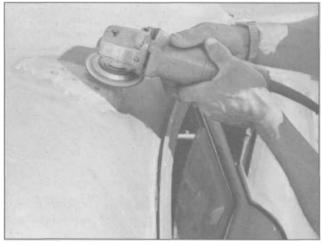
8.38 After the pulling, the stud heads are easily ground off without distorting the metal, and there are no holes left to fill in, as with conventional methods.
