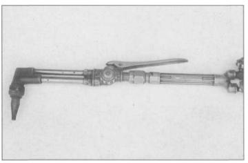
3.41 The cutting torch is adjusted for a good flame, then checked with the extra-oxygen supplied when the cutting lever is depressed. The flame should remain close to neutral. The excess oxygen is what is used to push the molten slag from the kerf as you cut.
