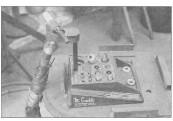
6.26 Spare, sharpened tungstens should be kept handy. This is a TIG caddy, which holds extra tungstens as well as spares for all your torch parts and different size collets and nozzles. The caddy is magnetic, and features a convenient torch rest.
