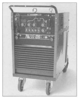
6.12 When you go up in welding machine size, you get more amperage and higher duty cycles. This TIG-Star 250 operates on several single-phase input currents, and has a 60% duty-cycle at 200 amps, with 100% duty-cycle at 140 amps.
