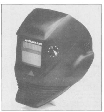
8.6 This Darth Vaderish design from ESAB is the Autorama 2000, which one of a modern breed of welding helmet with an automatically-darkening lens. The lens is powered by solar cells, and turns dark as soon as the welding arc begins. These are considered by many weldors to be much easier to use than flipping a helmet up and down to set up each weld.
