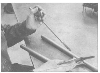
6.38 In use, the Pocket-Feeder can be used with either left or right hands, and you can reload new wire with one hand. Sensitivity on the thumbwheel is good, even with a light glove on.
