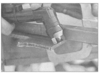
7.22 Same tool as the previous photo, showing how it holds the tip away from the work, and provides a good surface to lightly drag against your pattern or straightedge.
