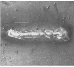
5.44 This is what some of your practice welds will look like. The heat setting was too hot here, and the weldor wasn't very steady with the gun. Use both hands and find a very comfortable position to hold it steady. Note the amount of spatter from making and breaking the arc.
