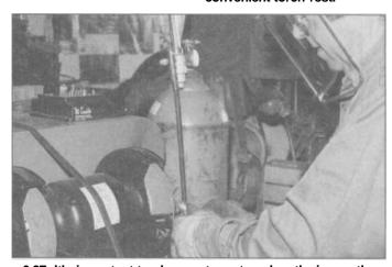
6.27 It's important to sharpen tungstens lengthwise on the tip, so as not to leave any radial grinding marks that could cause arc scatter. Grind points for steel like a pencil, like a crayon for welding aluminum.
