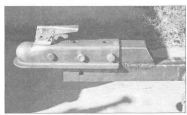
9.34 We originally had the hitch bolted to the main tongue, but found we had a better tongue weight with the tongue down another two inches. Simply welding on another piece of 2x2-inch, heavy-wall tubing set the trailer just right.
