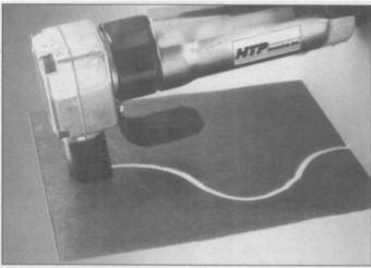
8.32 An air-powered "panibbler" is a fast, clean way to cut sheet metal up to 3/64-inch in steel or 5/64 in aluminum. It will follow a pattern or cutline very closely, and you control the speed with the throttle. This one is from HTP.
