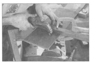
7.20 The plasma cutter makes very clean cuts, so any raggedness on yours means your hand wasn't steady. Use a sturdy guide whenever possible. With a piece of tubing as a straightedge, here a dry run is being made to ensure the torch follows the correct cut line.
