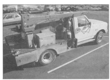
1.11 Not every welder and weldor works indoors. This is an oil field service truck with gas-welding/cutting equipment, arc welder and crane. Many welding shops have portable setups like this for remote jobs.
