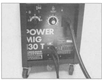
5.6 There are very few user controls on the panel of a basic MIG welder, just a switch for the different amperage settings, and a variable knob for controlling the wire-feed speed.
