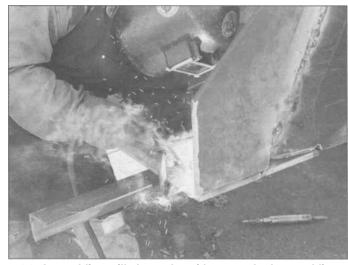
4.1 Arc welding will always be with us, as the best welding method for joining heavy plates for commercial, farm and industrial work. The weldor requires considerable protection from the spatter and radiation, usually wearing heavy leather protective gear.
