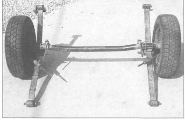
9.4 Bolt your springs, U-bolts, spring plates and shackles together, making sure the springs are square to the axle centerline and measuring the same distance apart front and rear.
