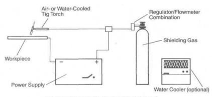
COMPONENTS OF A TIG WELDING SYSTEM
