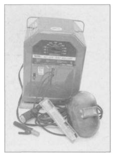
4.2 For home and farm use, the Lincoln 225 is the classic AC buzz-box welder, having been in production relatively unchanged for decades. Most home/shop units are AC only, and require some rewiring to accommodate the required 220V input.
