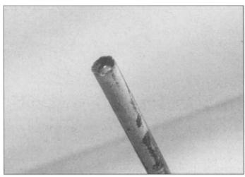
4.25 Some arc rods melt the wire at a faster rate than the flux, leaving the wire recessed inside. During the welding, this makes a more concentrated arc spray. When re-striking an arc with such a rod, the extra flux around the tip must be broken off with your gloved fingers or pliers (with the rod cooled off) to expose the metal for re-striking the arc.
