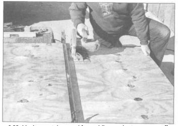
9.28 Having metal around for welding projects can pay off when working with wood, too. Use an extra length of straight angle-iron or tubing to clamp down on a piece of plywood as a saw guide, for perfectly straight cuts.
