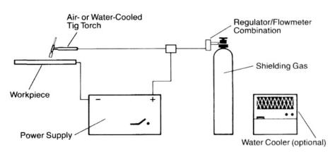
COMPONENTS OF A TIG WELDING SYSTEM
