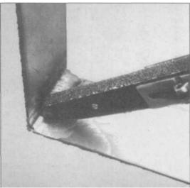
8.26 HTP is marketing this clever belt-sander that can get deep into corners and places where regular sanders and grinders can't reach. The belt guide rotates 160 degrees, and the sander uses 3/8-inch belts.
