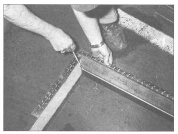
9.13 We used what materials we had, with 2x3-inch tubing for the two main rails and 2x2-inch tubing for the rest. When joining tubing of different sizes, cut one to a standard 45degree angle (here the 2x3), then lay the next piece in, square it and mark along the second tube for the correct angle to cut it.
