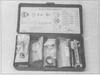
7.19 You'll need to keep on hand some spares of each of the torch components, including wrenches for changing the tip and the electrode.
