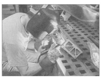
6.4 Unlike arc-welding or MIG-welding, the weldor can get very close to his work with heli-arc equipment. Even when welding on this cast-aluminum dry-sump oil pan, smoke is minimal and the arc not nearly as intense.
