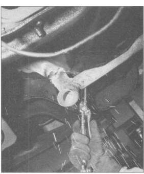
3.40 Sometimes, the oxy-acetylene cutting torch the fastest, easiest way to remove the old exhaust system.
