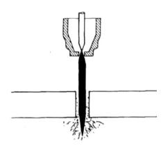
7.4 In plasma-arc cutting, there is usually only one gas (in all but the biggest machines), and that is air from the shop's air compressor, which is forced around the electrode to blow the kerf out neatly.
