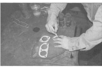
7.25 Here an exhaust gasket is being traced to make thick header flanges from a piece of 3/8-inch steel plate.
