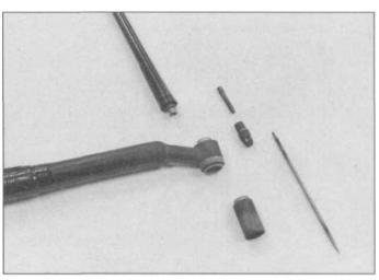
6.9 The exploded view of the typical TIG torch shows the tungsten (right) and from top to bottom: the back cap, collet, collet-chuck, torch body, and ceramic cup or nozzle. To assemble, the collet-chuck is screwed into the torch body on the bottom, the nozzle is screwed in on the bottom, the collet slides in from the top, and then the tungsten is slid in and retained by the back cap.
