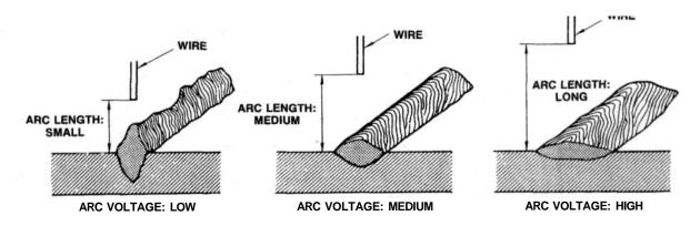
5.49 Arc voltage and length affect the shape of the bead's profile and its penetration. Cut a few of your practice welds in half to examine the beads. The shape of the overlapping puddles should have rounded ends exposed, not sharp, triangle ends.
