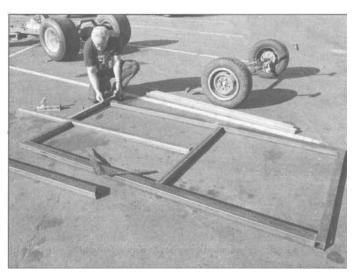
9.12 If your driveway or shop floor is flat enough, lay out your pieces of tubing on the ground and check all your measurements. Cut your joint angles carefully, and, with the pieces laid out, measure diagonally from corner to opposite corner to see if the frame is square. Check this again several times during the tacking and welding phase, too.
