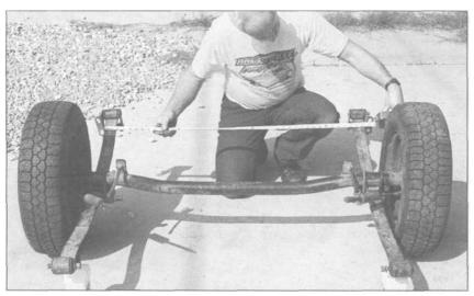
9.6 In our case, we determined that the Sprint axle was too narrow for our purposes, since we wanted a full 4x8-foot sheet of plywood as a floor. This meant widening our tubular axle 7 inches.
