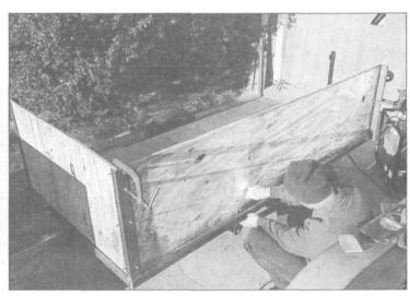
9.31 Plywood sides are bolted to the end pillars and the side plates.
