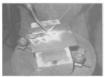
3.35 You should start with very clean metal when brazing, although the flux is designed to surface clean as you go, leaving some minor slag afterwards. You will have to keep the torch further away from the seam than with welding, to keep from overheating the brass.
