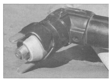
7.21 This clever tool snapped onto a Miller plasma torch holds the torch just the right distance away from the work, so if you have this and a sturdy guide, your cuts should be almost as good as machine-operated torches.
