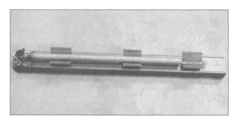
8.42 Leftover pieces of tubing and other stock should be saved in a barrel. You never know when you need a short piece. This fixture for making up a street rod four-link rod is made from short pieces of angle-iron and a length of rectangular tubing.
