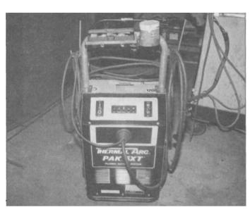
7.18 Hot rodders never leave anything alone. Rugged Thermal Dynamics 50-amp plasma cutter used in a rod shop has been modified with the addition of a tubing rack and box on top to hold nozzle dip and plasma consumables.
