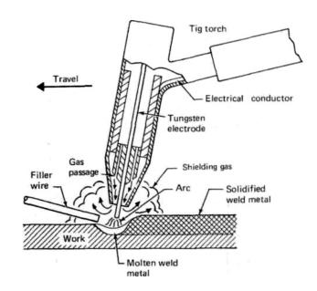
6.1 The **TIG** process is considered the most precise, most controllable and cleanest method of welding. The arc is made between the work and the central tungsten electrode in the torch, while a flow of shielding gas comes in from the nozzle. **Note** the low angle of filler rod addition. TIG or heli-arc **welding** is also one of the most observable welding process, with no spatter and little smoke.
