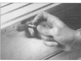
8.30 For small jobs, Eastwood offers these little Cleco-type panel holders that you operate with your fingers. No tool is needed. They have a range of up to 1/4-inch for thickness and fit a 1/8-inch hole.
