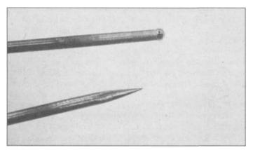
6.28 The tungsten at bottom has been sharpened for use on steel, while the top one is for aluminum, with a small ball-shape on the end. In theory, you could create a ball-end like this by striking an arc on a piece of copper before using the tungsten on aluminum, but a suitably-dull point will turn into a ball like this with a few seconds use on HFAC for aluminum.
