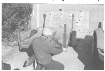
9.27 Four posts of heavy 1x2-inch angle-iron were welded on, one in each corner, as supports for the plywood sides.
