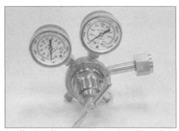
3.19 Most home/shop users of oxy-acetylene will have single-stage regulators on their torch sets. Unless you do a lot of welding/cutting, these are just fine, though you have to readjust the output pressure more frequently than with the professional, two-stage regulators.
