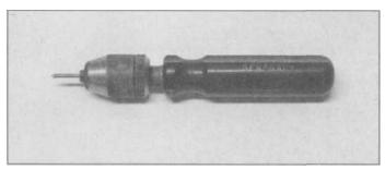
6.25 Make the most of expensive tungsten electrodes by using them until they are too short to fit the torch'. Shorter tungstens can be safely sharpened without burning your fingers, using a tungsten-holder like this.
