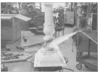
3.54 The rosebud tip will be useful for heating metal parts to be bent, freeing press-fitted parts, and for preheating castings before welding, such as here where a cast-aluminum mailbox post is preheated before TIG welding.
