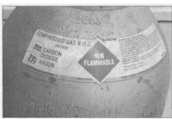
5.33 Most of your welding with shielding gas can be done best with a 75% argon/25% CO<sub>2</sub> mixture, which is excellent for cleanliness and penetration, and can be used on cast-iron and stainless-steel as well.
