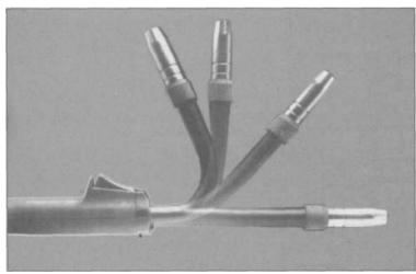
5.58 For tight quarters such as muffler work and other roundtubing situations, HTP makes this MIG gun with a flexible swan neck. It can even be used straight ahead, to reach into a spot where you can't get your hands.
