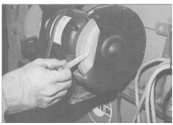
7.24 As with traditional torch cutting, soapstone is useful to mark your cut lines because it won't burn off. With the reduced heat of plasma, you could also use a marker pen. Sharpen the soapstone before drawing.
