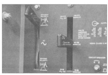
6.23 The lever at left on this Miller TIG sets the polarity, while the right lever is the coarse amperage, with a bottom setting of 10-55 amps, a medium range of 40-190, and a top range of 125-310 amps. Within each range, the fine-amperage knob sets the upper limit for the pedal.
