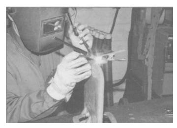
2.24 While TIG or heli-arc welding is considered by many to be the most controllable welding technique, it takes more practice than any other. You have to learn to manipulate the torch with one hand, the rod with the other, and the amperage control with your foot on a pedal. There are no sparks, spatter or slag. Here an aluminum frypan's handle mount is being repaired. The heli-arc welding didn't even bother the non-stick coating on the other side!
