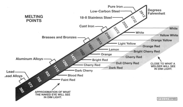
2.2 Welding is a process of *fusion*, in which metal parts are heated to the melting point and fused together, usually with a filler of the same material melted along with the "parent" metal. All metals melt at different temperatures, and this chart shows some interesting comparisons, as well as relating the heated metal's color to its temperature.
