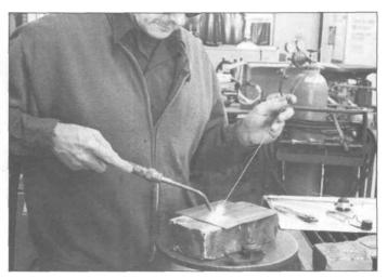
Butt weld Deposit
