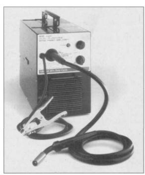
5.19 There are small MIG machines that come equipped for use with flux-cored wire, but have an optional kit that can be attached to work with shielding gas and solid wire. Eastwood Company's wire-feeder uses 110V current, and has a 20% duty-cycle at its maximum amperage of 85. It's fancooled and adequate for light-gauge welding.
