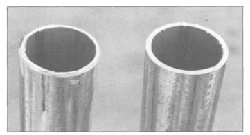
9.8 This axle is heavy-wall tubing, and, since we wanted good weld penetration for strength, the cut ends were beveled with a grinder. Tube at left has been beveled to about half its thickness.
