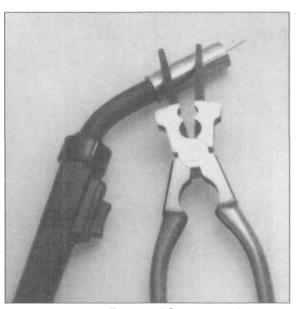
5.12 Eastwood Company makes these multi-function **MIG** pliers, which can be used to clean nozzles, snip wires, and hold contact tips to unscrew them.
