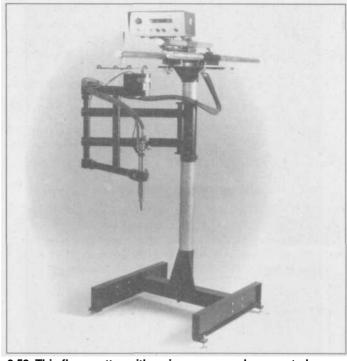
3.52 This flamecutter with swing arms can be mounted over a plate, or bolted to a table.
