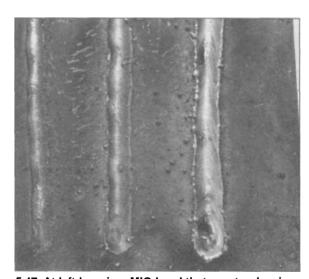
5.47 At left here is a MIG bead that was too low in amperage for the thickness of the material. Penetration is shallow and the bead sticks up too high. At center, the correct amperage was used, and at right, the amps were too high. The right-hand bead may look OK here, but penetration was too deep (dropthrough on the backside) and there was some undercutting on either side of the bead.
