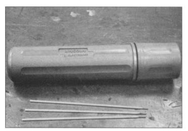
4.28 Rods must be kept dry for the flux coatings to work properly. Keep only as much rod as you need, and store them in a tight container such as this Lincoln plastic rod box with gasketed screw cap.
