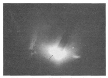
4.12 This is what you will see through your helmet and welding lens. The arc is intensely bright, but the lens cuts this down to just a bright glow around the arc itself, here you can just about see where the shielding gas cloud forms around the arc.
