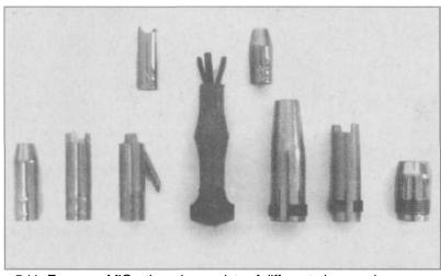
5.11 For some MIGs, there is a variety of different-size nozzles, some with special purposes like spot-welding. At the center here is a tool for scraping debris from inside a nozzle.
