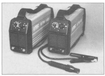
4.29 These L-TEC portable arc power sources are lightweight, and offer up to 90 amps on the STW 90i (right) and 130 amps on the STW 140i. Unlike most small arc welders, these are DC, and can even be set up with a torch and power adapter to run a TIG torch. They are available for 110V or 220V input.
