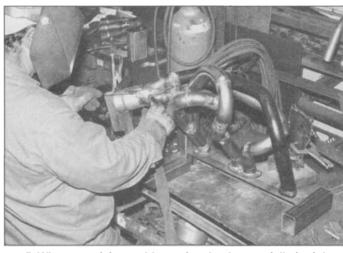
6.5 Where precision welds are involved, especially in tight quarters such as on this stainless-steel race-car header, TIG welding's wide range of operator control is seen as an advantage.
