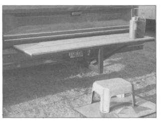
5.61 You'll find many uses for your welder once you get used to using it. This example of a typical home project is a plywood-covered rear bumper extension for a truck. It's used for carrying extra camping gear, and used as a tailgate for working or cooking when camping. Its also a wide step when stepping out of a camper shell on the truck.
