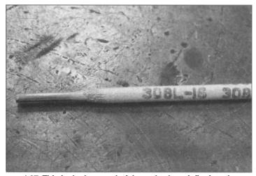
4.27 This is the bare end of the rod, where it fits into the electrode holder. You can judge the size of a rod from this bare end - don't measure the flux coating. Rods are marked as to their type and color-coded.
