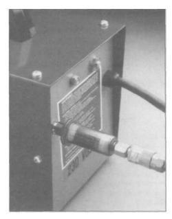
7.26 The 50-amp plasma cutter makes short work of cutting out the patterns and can easily pierce the center of a pattern to cut out internal holes and shapes.
