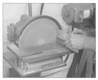
8.24 A disc sander with at least 1/2 horsepower is very handy around the shop for squaring edges of flamecut parts, and taking sharp edges and corners off work.
