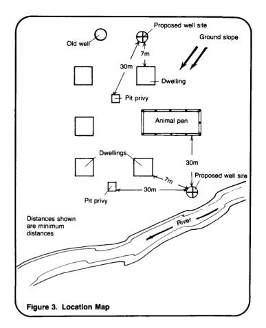
To summarize, give the construction foreman a location map similar to Figure 3, described in "Selecting a Well Site," RWS.2.P.3, design drawings of the method of casing installation similar to Figure 1 and the type of screen similar to Figure 2a, b, c, d, or e, and a detailed materials list similar to Table 1.
