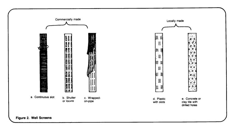
Commercial Screens. Probably the best commercial screen is the continuous-slot type, which consists of a triangular-shaped wire wrapped around an array of rods. The screen offers the largest percentage of open area for water to enter, while retaining a small slot size to screen out particles. Another advantage is that the triangular-shaped openings prevent particles from sticking in the screen and clogging it. The size of the slots can be precisely regulated and can be as small as 0.15mm.
