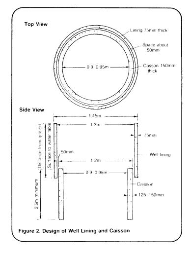
Often, both methods are employed in a single well: dig-and-line is used until the water table is reached, then caissoning is used to sink the well into the aquifer. The lining is usually 75mm thick and the caisson rings are 125-150mm thick. The outside diameter of the rings is 50-100mm less than the inside diameter of the lining to allow the rings to freely move downward. Table 1 shows common dimensions of shaft, lining, and rings.
