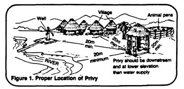
• Be sure that the pit does not puncture an aquifer. Latrine seepage that enters an aquifer can contaminate ground water (wells) and spring water supplies.
