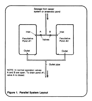
Figures 1 and 2 show two pond system layouts. When the layout has been determined, prepare a drawing similar to one of the figures showing the arrangement of ponds, and the type, width, length, and depth of each pond. Give the drawing to the construction foreman.
