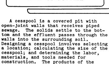
design process are: (1) a location map, (2) a plan view of the cesspool, and
