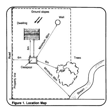
When an acceptable site for a cesspool has been found, draw a location map similar to Figure 1, showing distances from the site to water supplies, dwellings, property lines and trees. Give the map to the construction supervisor before construction begins.
