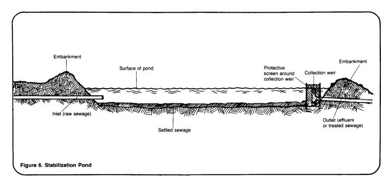
Stabilization pond systems, shown in Figure 6, use a large sewer main pipe to carry the collected sewage to the inlet of the pond. The pond is normally 1m deep and its surface area is large enough to provide a predetermined time for treatment. An average-size pond is 15m wide and 30m long. The treated sewage is continually and slowly drained off to assure the proper retention time.
