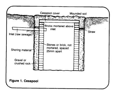
The <u>inlet</u> is the end section of sewer pipe which carries sewage from a building to the pit. The pipe and inlet are usually 100mm in diameter.
