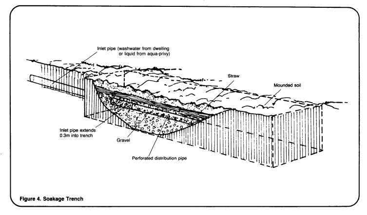
Soakage trenches are 0.6-1m wide, 0.6-1m deep, and vary in length from 6-30m depending on the quantities of washwater and the permeability of the soil. The bottom of the trench must be at least 1m above groundwater levels, and it must slope gradually downward away from the inlet end.
