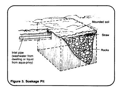
with dirt. The gravel prevents the sides of the trench from collapsing and allows washwater to flow through and drain to the bottom of the trench. distribution pipe is not available, concrete blocks can be used instead. The straw prevents soil from sifting down and clogging the flow of wash-The pipeline carries washwater water. from a sink or drain in the dwelling, or excess liquid run-off from an aqua privy. The pipe extends into the higher end of the trench.
