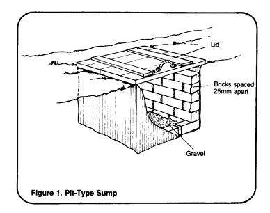
Washwater is poured directly into a sump and gradually soaks into the ground. Sumps are to be used only where there are 5 liters or less of washwater per person per day. Larger quantities of washwater require a soakage pit or soakage trench.
