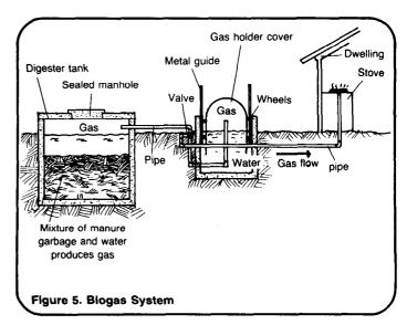
The digester tank and the bottom and walls of the gas holder are usually made from reinforced concrete. The cover of the gas holder is made from sheet iron and, because of its strict design specifications, is either purchased as a prefabricated unit or made in the community by skilled craftsmen. Gas pipes and valves must be purchased.
