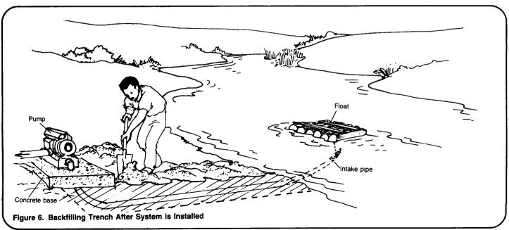
8. Install the pump. For information on pump installations, see "Installing Mechanical Pumps," RWS.4.C.2, or "Installing Hand Pumps," RWS.4.C.3. Use "Constructing Dug Wells," RWS.2.C.1, in constructing a storage well. Figure 6 shows the connection of an intake pipe to a pump.
