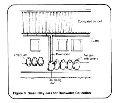
A similar technique is to use smaller, portable clay jars that can easily be moved under the downspout during a rainstorm. A family could have several 25-liter jars which can be filled during rainfalls. This system will work efficiently, but there will be little storage capacity for the dry months.
