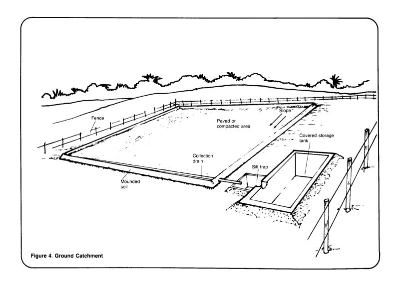
Materials. The ground catchment surface is very important in collecting rainwater efficiently. Catchment surfaces must be impervious to avoid water losses from infiltration and seepage. On pervious surfaces, much of the rain will be lost for community use. Part of it will wet the ground and part will be stored in small ground depressions; other water losses will occur through infiltration into the ground, evaporation into the air, and transpiration through plants.
