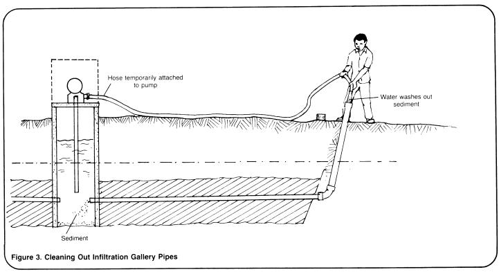
3. If the pipes remains clogged, it may be necessary to locate the clogging by digging out around the collection pipe. Begin digging at the point furthest from the well and dig toward the well. Uncover the entire collection pipe and locate where the clogging is occurring. Clean those areas. Use buckets of water from the well and flush out the sediment from the system. Lay fresh sand and gravel in the filter bed before backfilling the trench.
