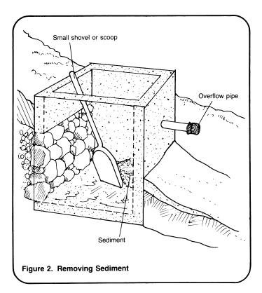
Check the screening on the pipes to see if cleaning is necessary. If screens are clogged or very dirty, they should be either cleaned or changed. Always use copper or plastic screening to prevent rust.
