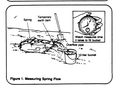
leakage around the pipe. Then, put a bucket of a known volume (for example, a 10-liter bucket) under the pipe to catch the flow. With a watch, measure the amount of time it takes for the bucket to fill. Divide the volume of water by the amount of time to find the rate of flow in liters per minute. For example, if the 10-liter bucket fills in 45 seconds, the rate of flow is:
