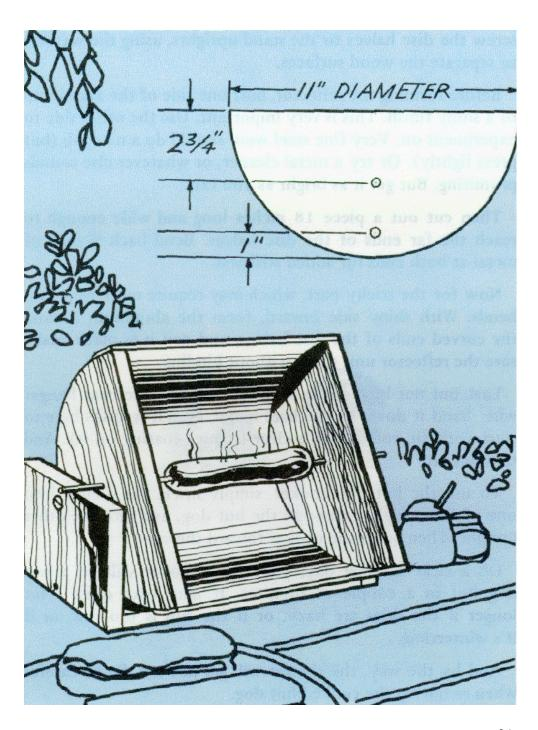
Next comes the support stand. In each short piece of wood, drill a hole one inch from either cut end and halfway between the sides. Make the hole slightly larger than the diameter of the wood screws. Then nail the short pieces to the ends of the remaining piece of wood to complete the stand. Finally, screw the disc halves to the stand uprights, using the washers to separate the wood surfaces.
