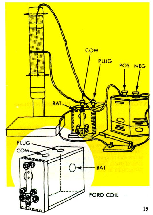
OK, let's see what our smoke trap can do. Hold a source of smoke under the bottom of the "chimney." A burning incense cone or twisted damp paper towel should work nicely. When you see smoke coming from the top of the chimney, close the knife switch. Hey, it works! Now open the switch to see if the chimney starts smoking again. Yup, there it goes. Naturally, your model won't be as efficient as industrial electrostatic precipitators. But its principle will certainly be the same.
