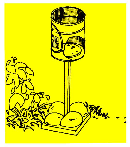
Another method would be to put a large saucer of clean water in the coffee can instead of the cardboard. Actually, you won't need the saucer if the nail hole in the bottom of the can doesn't leak. Keep adding water from time to time to make up for evaporation losses. After a few weeks, let all the water evaporate. Then check for the dirt.
