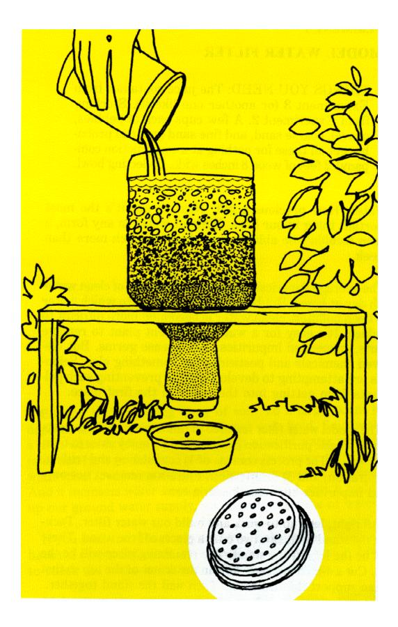
Using a sharp instrument (easy there), slice the very bottom off the plastic container. Next, we want to convert the cap, minus the liner, into a screen. So with either a 1/16-inch drill or a pointed tool, make as many holes as practical in the cap, then cover all the holes with a piece of stocking. Screw the cap back on the container, and seat the container upside down in the stand.
