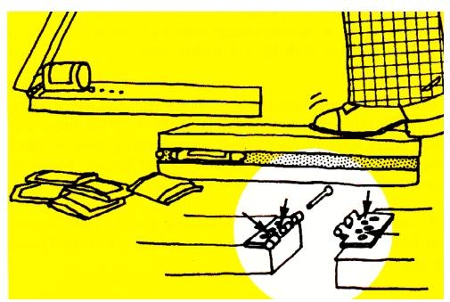
Your crusher will only be as strong as the hinge you use. So the huskier the hinge, the better. Position each hinge plate on the boards as shown in the drawings (you don't have to take the hinge apart to do this). Note that the hinge-pin loops extend beyond the board edges. Also be sure the countersunk screw holes are facing upward.
