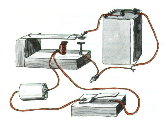
A MESSAGE COMES IN. Note that when the low-voltage telegraph key is depressed (from miles away, remember?), the nail becomes an electromagnet and pulls the strip down. This closes the higher-voltage circuit, lighting the bulb. When the key is released, the electromagnetic field collapses, the strip springs upward, and the bulb circuit opens.
