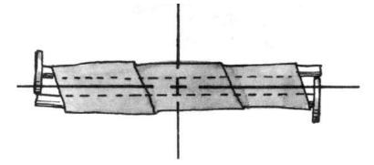
We will be putting on four layers of wire. Begin right next to the shaft. Leaving some wire for circuit connections, wind neatly toward the nail head. Keep each turn of the wire close to the preceding turn. Upon reaching the nail head, double back toward the shaft. Then make another trip to the same nail head, and return again to the shaft.
