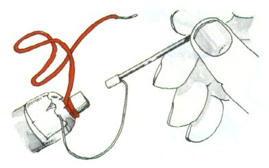
INSTALLING THE LOCK. Cut a metal strip 3" by 1-1/2", and form it around the coil. Bend the ends outward, and punch two holes in each end to receive the nails. Before mounting the lock, ener-
