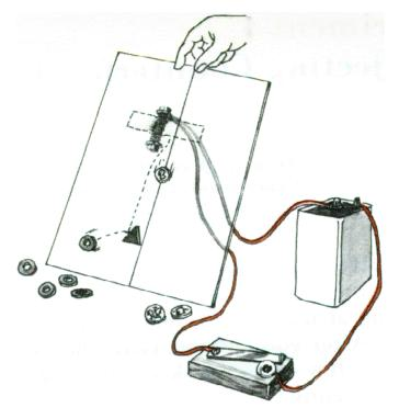
centerline, let several coins and slugs (washers) slide down the cardboard. If our slug rejector is working properly (bet you forgot to close the switch), all the slugs will be attracted to the electromagnet side of the divider, and all the coins will drop straight down . . . somewhat like in Edison's ore separator.
