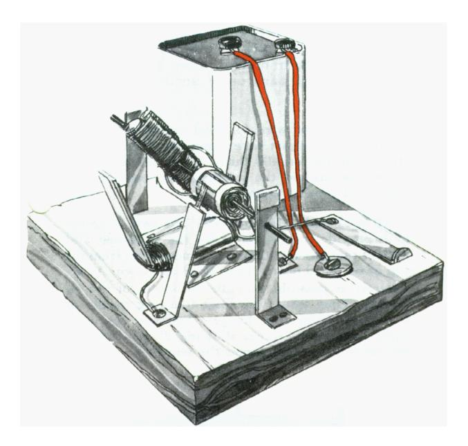
Materials: Strap iron 6" by 5/8" by 3/32" (or 1/8") 100' of. #24 magnet wire. Two 16-penny spikes. Tape 1" wide. Daring needle or piece of coat hanger. Various metal strips. Copper-strand lamp wire 2" long. Baseboard 7" by 6" by 3/4". 4 screws. Some nails. 1' hookup wire. 6-volt battery.
