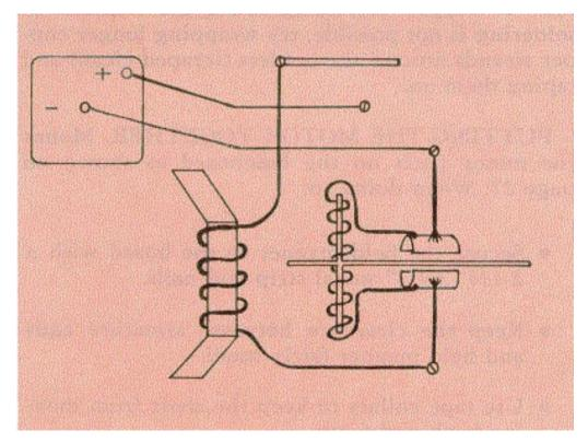
OK, START HER UP. Ready for the big moment? Let's keep our fingers crossed as we close the switch. You may have to give the armature a little push. If all the connections are good and nothing is binding the shaft, the motor should spring to life. Try adjusting brush pressure for better performance. A little oil in the shaft support holes will help too.
