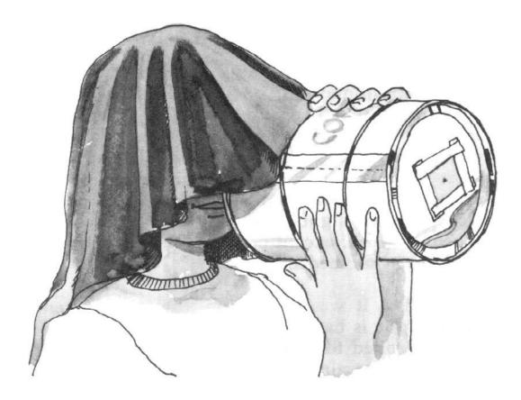
SCREEN AND LIGHT SHIELD. The plastic lid is our viewing screen. However for you to be able to see the projected image of what you aim at, the screen has to be shielded from light. For this purpose, drape the dark cloth over your head and the camera, the way some photographers do.
