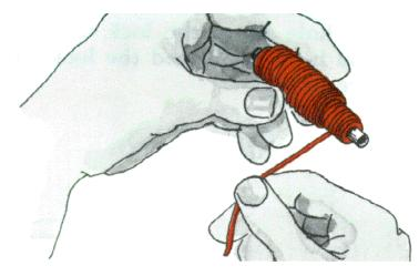
ROD AND SUPPORT. Make the rod by cutting a 2" section from the middle of the 8-penny nail and filing off any sharp edges. Then lay a 3" piece of elastic thread next to the rod, side by side. Tape them together at one end, as shown. Now lower the rod, taped end pointing down, into the tube until only 1/2" sticks out the top. Place the remainder of the elastic over the edge of the coil, and fasten it securely with tape.
