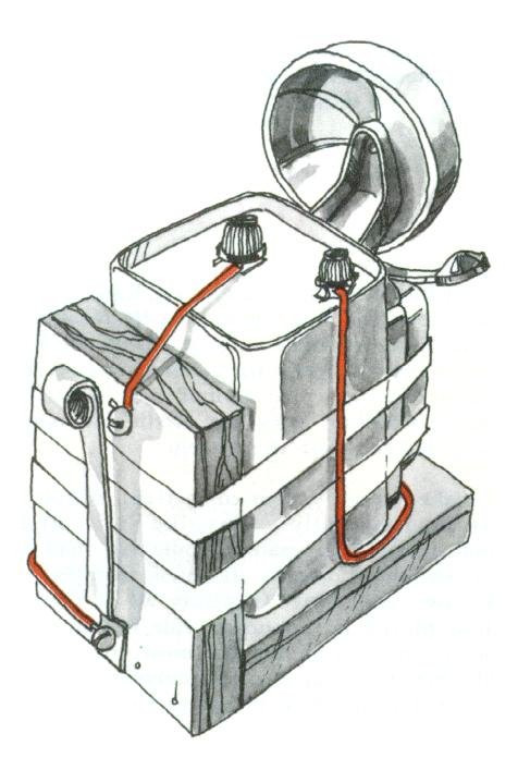
FINAL STEPS. Screw on the contact arm. Then complete these circuit connections: Run one doorbell wire to the battery, the other doorbell wire to the contact arm, and a third line from the upper contact screw to the battery.
