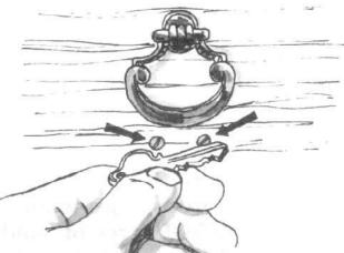
Anything metallic that can touch both outside terminals at once will be your "electric key." It could be a coin, a scout knife, a metal-edged ruler. Of course, touching the terminals and pulling on the drawer will have to be done at the same time. And it should be done quickly, to conserve the battery.
