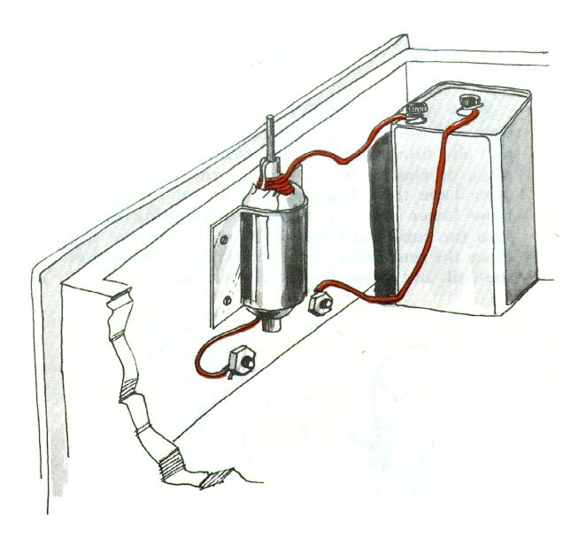
CONNECTING THE CIRCUIT. The battery and lock are connected in series with two terminals (machine screws) that come through the drawer from the outside. Wires from the coil and battery are attached to these screw terminals with nuts.
