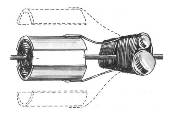
spaces should face the same direction the nails do. Put a thin strip of tape around each end of the commutator to keep it together. This completes the armature-commutator-shaft assembly. OK so far?
