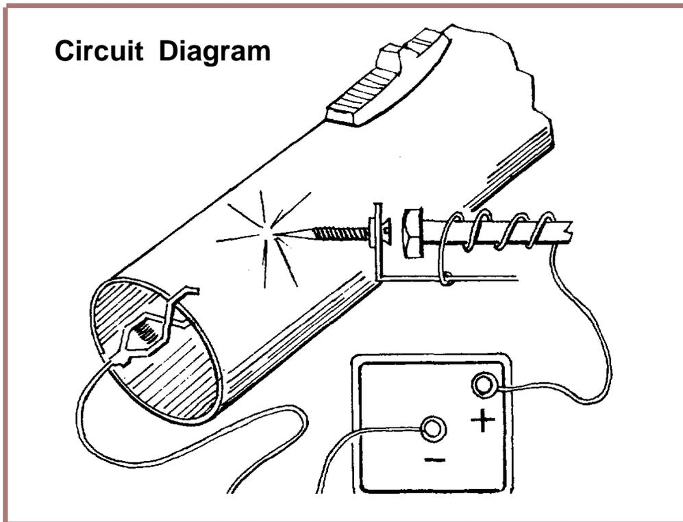
**BROKEN ARC STOPS CURRENT.** When the increasing distance between tip and flashlight becomes too great for the arc to continue, the arc breaks. Immediately, the magnetic field around the coil collapses, and the core releases its electromagnetic hold on the tip. Tension on the flexed metal arm then snaps the tip back onto the flashlight. And the cycle begins all over, repeating itself many times each second.
