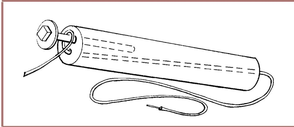
**FORMING THE ARM.** Fold the 1/2" by 3" tin-can strip in half, lengthwise, so that it measures 1/4" by 3". Doubling the tin-can thickness in this manner will give us the approximate flexing stiffness the arm needs. To fold the strip, simply scratch a line down the middle, clamp the strip in a vise at the line mark, and tap sideways with a hammer.
