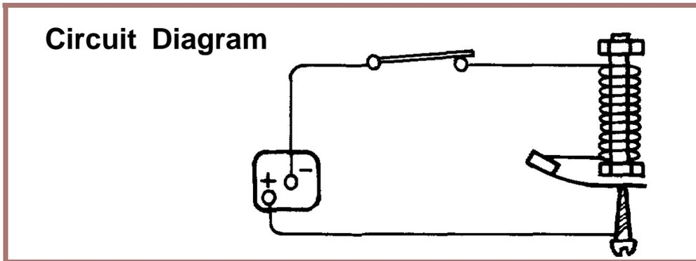
Instantly, current shoots downward to the brass contactor screw. Since the screw is touching the vibrator arm, the current continues on its way into the coil. Out of the coil it streaks past the closed code key and back to the battery.
