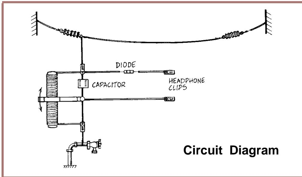
To get the most out of your crystal set, you must have a good ground connection and a good antenna. Cold-water pipes make excellent conductors to ground. Make sure the pipe has been sanded or scraped clean where you plan to make connection.
