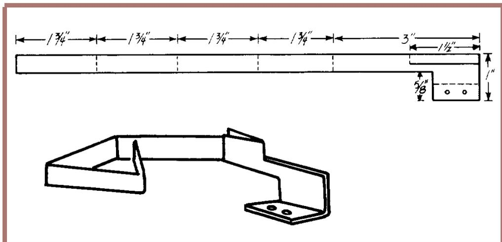
**FORMING THE VIBRATOR ARM:** Finish cutting and folding the 1" by 10" strip as shown in the drawings. Tap the folded ends with a hammer to keep the layers of metal close together. Punch two holes in the base so the arm can be mounted.
