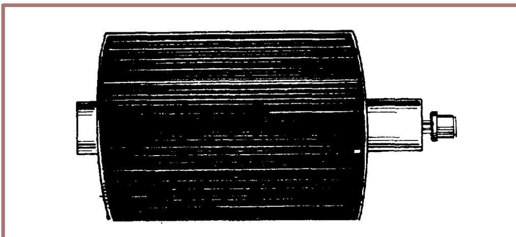
**THE ZINC ELECTRODE.** If you've managed to get a piece of zinc that is about 5" by 10", form it into a cylinder that just fits into the container you plan to use. The top of the zinc should be about 2" below the top of the container. Also, the zinc should have about a 6" length of copper wire soldered to it. If you don't have soldering equipment, pierce a hole in the zinc, thread the copper wire through it, and loop the wire around itself tightly.
