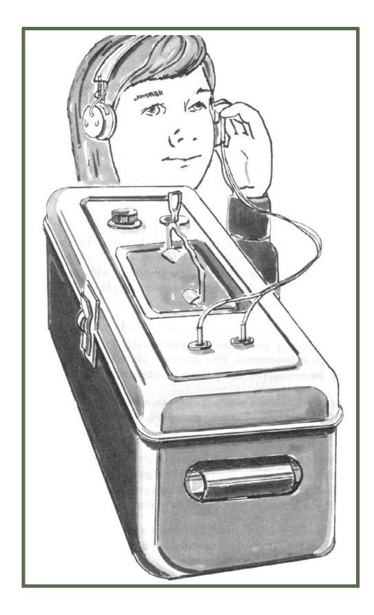
Some Geiger tubes will respond to alpha, beta, and gamma radiation. However, the tube we used has a thin metal envelope that cannot be penetrated by alpha particles. Thus, this instrument detects only beta and gamma rays, along with cosmic rays from outer space.
