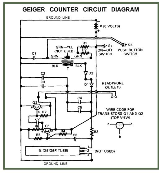
with your fingers. So mount it gingerly. Use "broom clips," one at each end. Also, make sure you connect to the right leads on the Geiger tube socket. The Geiger tube pins are numbered on the underside of the base. Pin 1 connects to the main circuit and pin 3 connects to ground. Pin 2 is a dummy pin that is not used.
