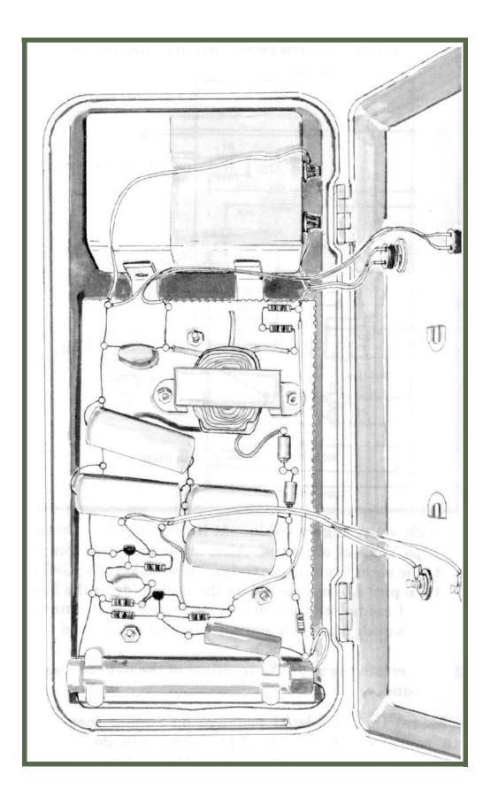
box, don't let any of the exposed wiring touch the metal walls.
