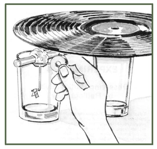
As soon as you bring the charged record into position, you will see the two foil leaves of the electroscope spring apart. They are reacting to the record's static electric charge.
