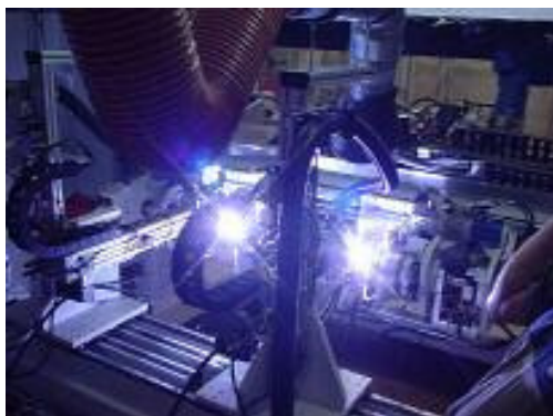
Fully automatic dual head welding- equipment for driveshaft, fillet weld
