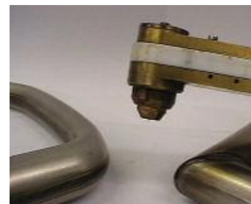
door handle made of stainless steel, no incursion of joint and no reinforcement of joint
