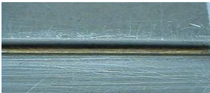
APN brazing: flange butt joint (view from above and micrograph)
