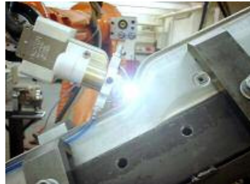
part of a vehicle/girder of ALMg3, 2x2,5mm-flange joint without additional material, v=2,5\text{m/min}
