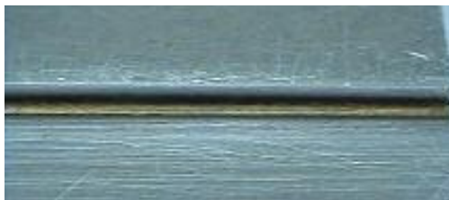
Brazing joint with CuSi3 solder on galvanised sheet, flange seem with overlaying border, v=3\text{m/min} without holes
