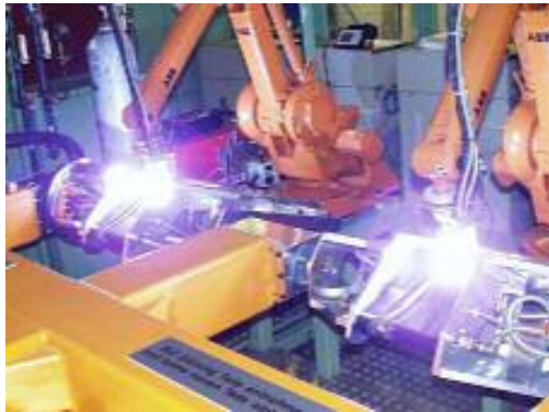
Safety part for a vehicle, hollow body out- of fine grain building steel, 2x1,2mm-flange joint, average v=2,4\text{m/min} . (higher speed possible)
