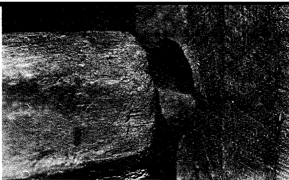
PLATE 282 This end of cloth beam is hewn into a knob to fit into hole in loom frame.
