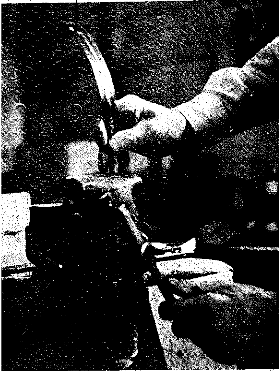
PLATE 10 Tedra places a piece of steel from a phonograph spring in a vice, clamping it at a point that allows the proper length for the knife blade.
