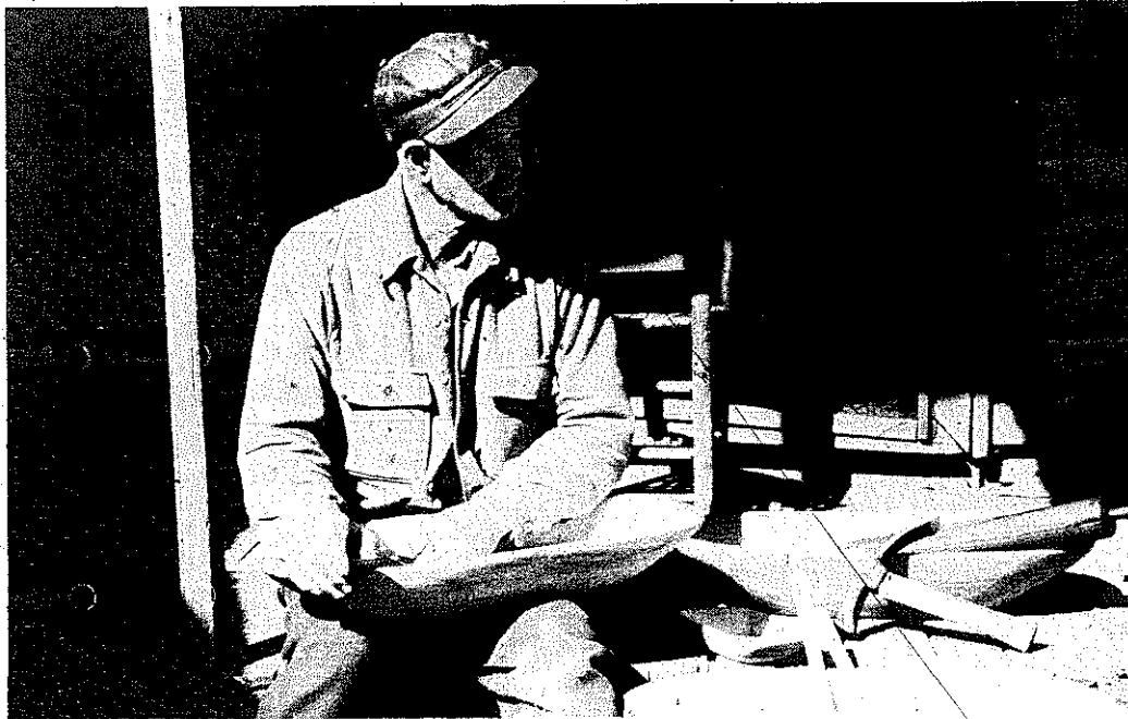
PLATE 109 Finally, using the hammer and chisel, Alex hews out the outside surfaces, and then does the final shaping and smoothing with a wood rasp and sandpaper.
