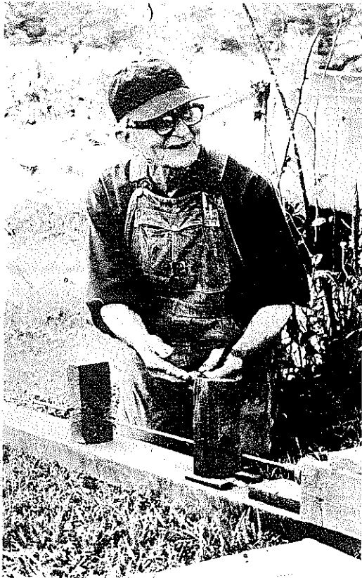
PLATE 192 To begin to rifle a barrel, Charlie pulls the guide back, inserts a barrel into the holes in the two blocks, wedges it into place, and begins to cut. The diameter of the metal rod closely matches the diameter of the barrel's bore. The rods are easily interchangeable depending on the rifle's bore.
