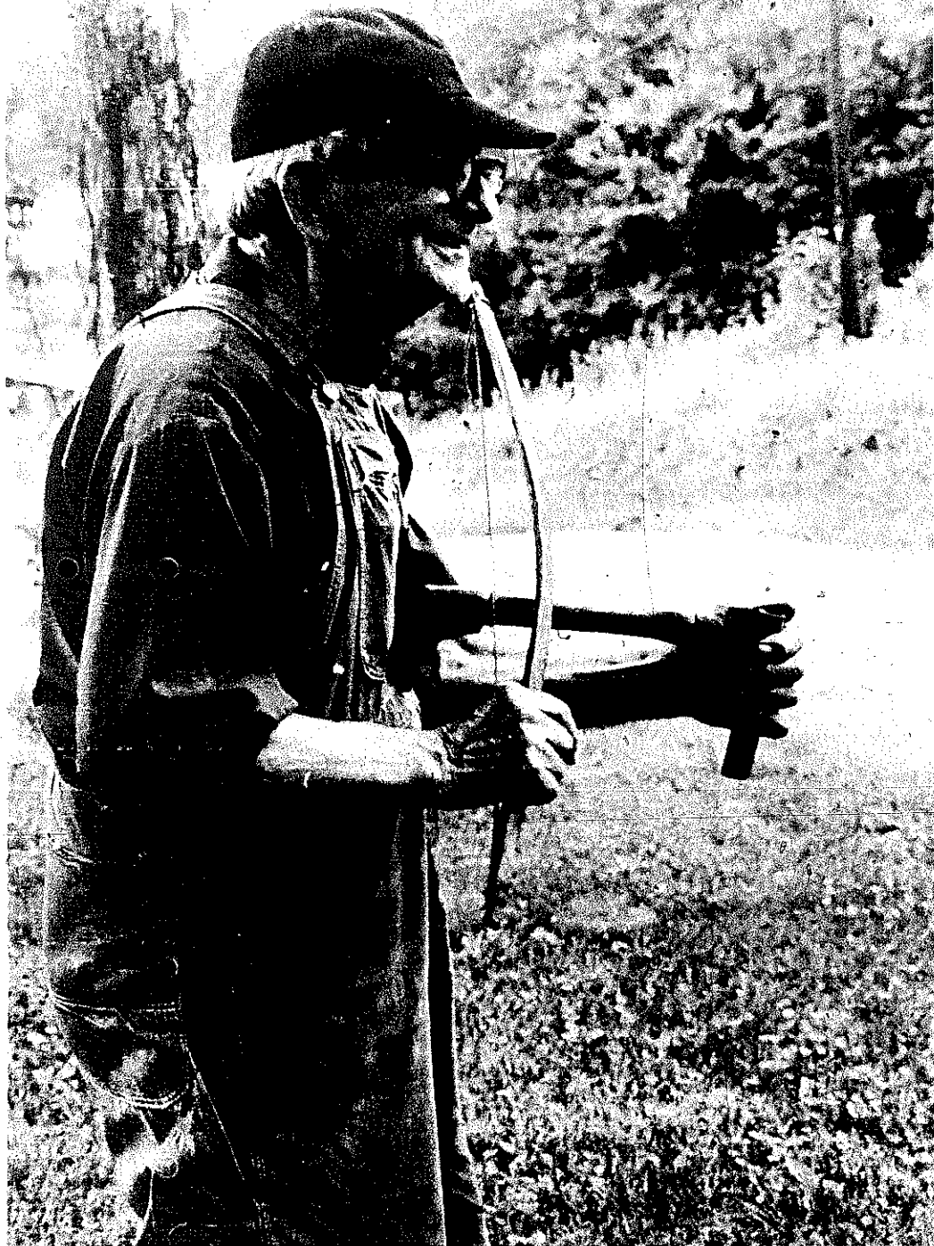
PLATE 194 In using his bow drill, Charlie often mounted the piece to be drilled (here held in his left hand) in a vise and then pressed the drill against it with his chest.
