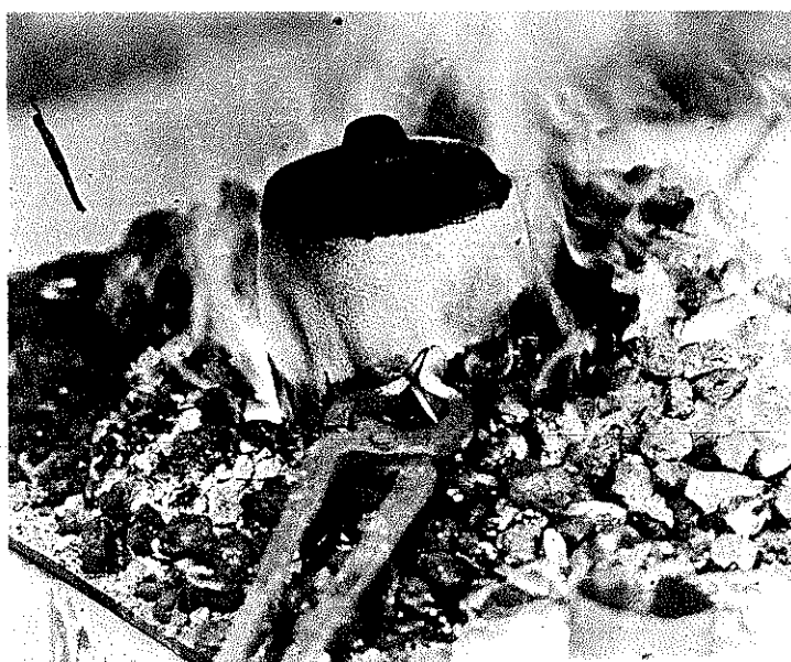
PLATE 198 Wallace Gusler tempering the lock in a crucible. (Photo courtesy of Colonial Williamsburg.)
