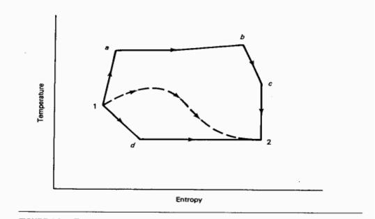
FIGURE 1.2 Two reversible paths and an irreversible path from state 1 to state 2.
