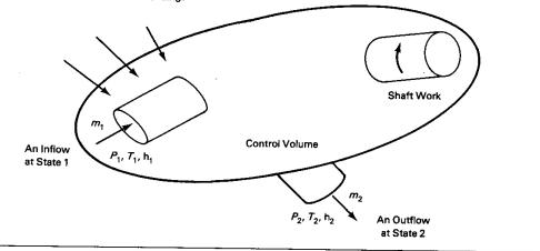
FIGURE 1.3 Control volume with an inlet and an outlet.
