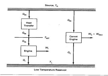
FIGURE 1.7 An engine model and a Carnot engine to determine the reversible work for the model.
