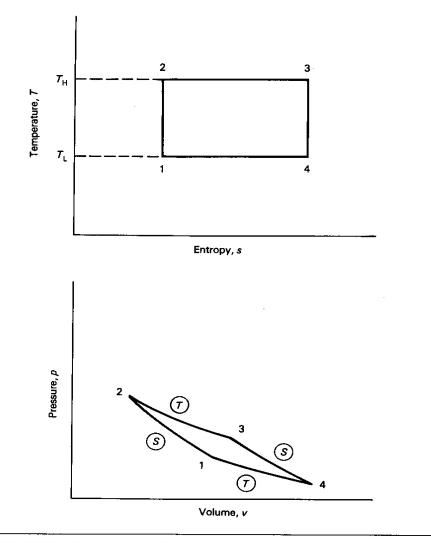
FIGURE 1.6 Carnot cycle, in T-s and p-v coordinates.
