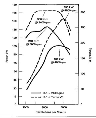
FIGURE 6.8 Comparison of normally aspirated and turbocharged 3.1-liter engines. (Reprinted with permission from *Automotive Engineering* magazine, October 1988. Society of Automotive Engineers.)
