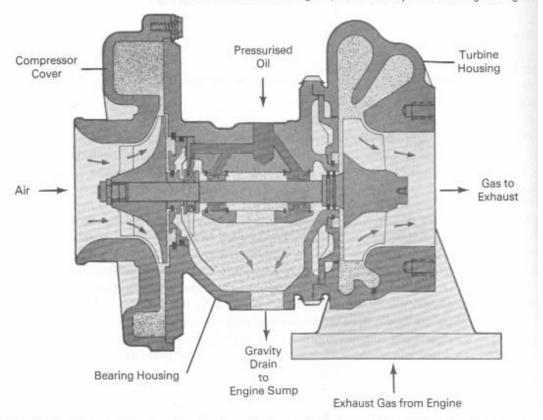
FIGURE 6.13b Cross-section of a diesel-engine turbocharger. (Courtesy of Holset Engineering Co.), Inc.)
