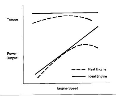
FIGURE 6.7 Torque and power characteristics of a reciprocating engine.
