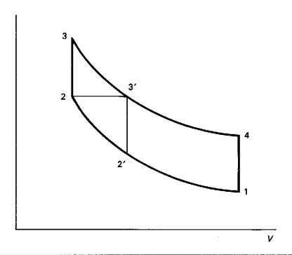
FIGURE 6.10 Comparison of Otto-cycle and diesel-cycle efficiencies.
