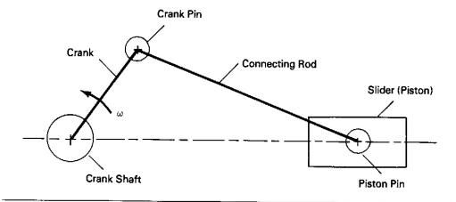
FIGURE 6.1 Crank-slider mechanism.
