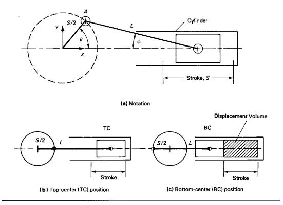
FIGURE 6.2 Geometry and notation for the crank-slider.
