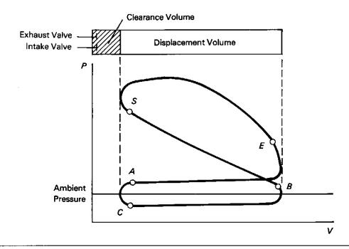
FIGURE 6.6 Indicator diagram for a four-stroke-cycle spark-ignition engine.
