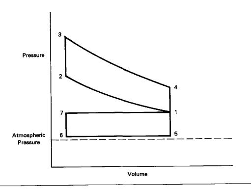
FIGURE 6.11 Supercharged Otto cycle.
