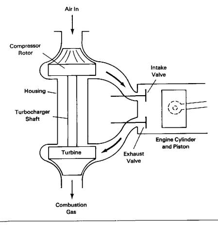
FIGURE 6.12 Schematic of a turbocharged engine cylinder.
