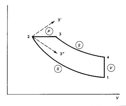
FIGURE 6.9 The diesel cycle.
