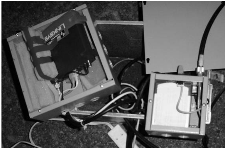
Photo 12-5: Inside the NEMA Boxes for the AP and Wireless Bridge
