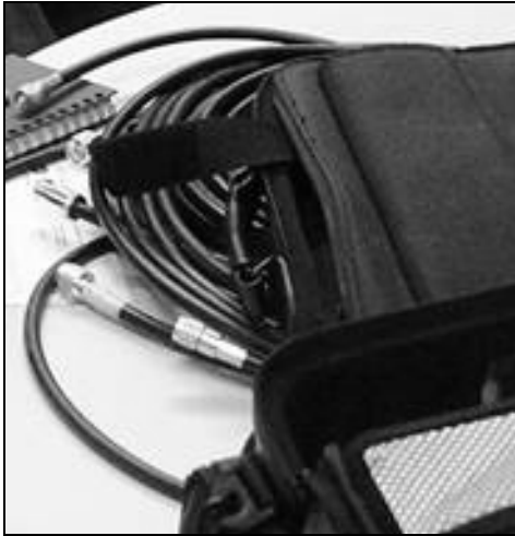
Photo 12-9: LNR 400 Coax Cable
