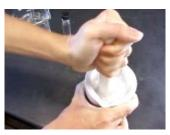
Grind about 2 grams of nanocrystalline titanium dioxide  $(TiO_2)$  in a mortar and pestle with a few drops of very dilute acetic acid. Alternate grinding and addition of a few drops of very dilute acetic acid (0.035 M) until you obtain a slightly soupy colloidal suspension with a smooth consistency.
