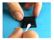
Wipe off the carbon along the perimeter of three sides of the carbon-coated glass plate using a cotton swab.
