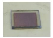
Heat the glass on a hotplate in a hood for 10-20 minutes. The surface turns brown as the organic solvent and surfactant dries and burns off to produce a white or green titanium dioxide coating. (NOTE: If the coating is too thick, it will crack and peel from the glass surface. If that occurs, allow the glass to cool, clean it, and recoat with a thinner  $TiO_2$  laver.)
