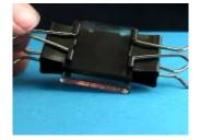
Assemble the two glass plates with coated sides together, but offset so that uncoated glass extends beyond the sandwich. Do not rub or slide the plates. Clamp the plates together.
