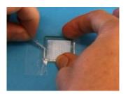
Carefully remove the tape without scratching the  $TiO_2$  coating.
