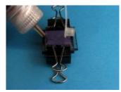
Add a few drops of a triiodide solution to the edge of the plate. Capillary action will cause the  $KI_3$  solution to travel between the two plates.
