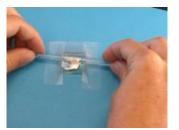
Add some of the titanium dioxide paste and spread using a glass rod. The tape serves as a 40-50 micrometer spacer to control the thickness of the paste layer.
