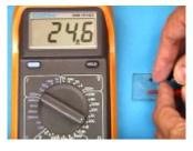
Identify the conducting side of a tin oxide-coated piece of glass by using a multimeter to measure resistance. The conducting side will have a resistance of 20-30 ohms.
