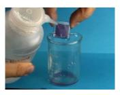
Rinse gently with water and then with ethanol. (The ethanol serves to remove water from the porous  $TiO_2$ .)
