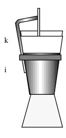
(See Franklin's figure 4 on previous page) In the early stages of understanding electricity, the mechanism of "storing electrical fluid" in the Leyden jar was not well understood. This experiment was actually an important one to show the conditions that could prevent charging the bottle.
