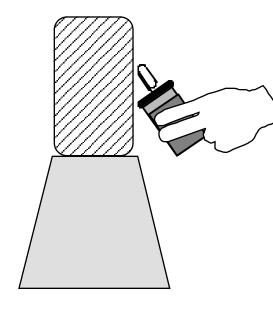
The diagram above shows electrification of a soda can repeatedly from the wire of the Leyden jar. Test for charge with the neon bulb. This experiment can be done as Franklin describes it, or simulated by using a soda can on a foam cup in place of the man on wax.
