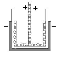
Here the Leyden jar has all of the normal amount of electrical fire that was on the outer coating transferred to the inner coating. I have not drawn the 20 plus signs and 20 minus signs that should appear
