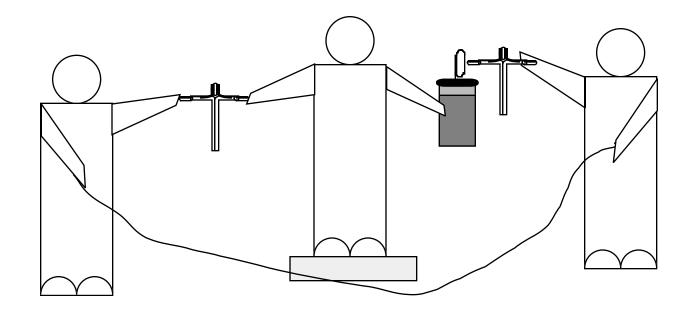
This is nearly a repeat of the previous experiment, but for Franklin it was important as some competing theories of electrification would have made a different prediction for the two cases.
