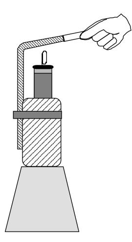
The diagram at right shows the attempt to electrify the soda can from the wire of the Leyden jar that rests on top of the can. Bend the foil covered straw down to touch the paper clip, holding only onto the uncovered part. Test the can for charge with the neon bulb, then test the Leyden jar for charge with the neon bulb.
