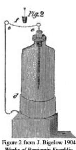
Figure 2 from J. Bigelow 1904 Works of Benjamin Franklin Vol II p. 200 (public domain) For this experiment, use a plastic drink cup Leyden jar. Fasten another foil coated straw to the outside with a rubber band, and fasten a bendy straw supporting a foil bit on a thread, so it can swing back and forth between the two foil coated straws.
