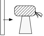
Franklin envisions the excess charge in the tube and the excess charge in the can as each having an electric atmosphere that extends some moderate distance from the object. These atmospheres push against each other, so moving the tube close shoves the atmosphere of the can which moves more of the associated electric fluid and its atmosphere into the tinsel, shoving the tinsel leaves farther apart.
