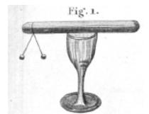
Detail of similar experiment using cork balls suspended from an insulated conductor.
