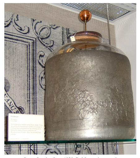
A large Leyden jar of the sort Franklin used to try to kill a turkey by electrocution. This one would have a liquid capacity of about 6 gallons. Franklin used a number of these connected together to form what he dubbed an "electric battery", as shown in the figure below.
