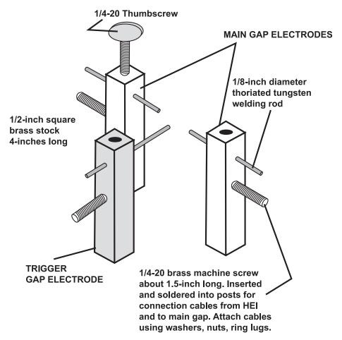
1. Cut three, 4-inch lengths from 1/2 square brass stock. Face each end of the length flat using a grinder or a hand file with a guide.
