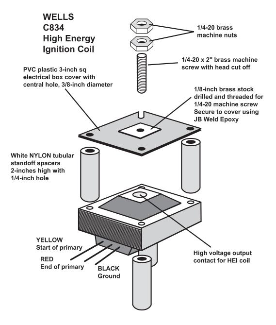
CONSTRUCTING THE SPARK GAP ASSEMBLY
