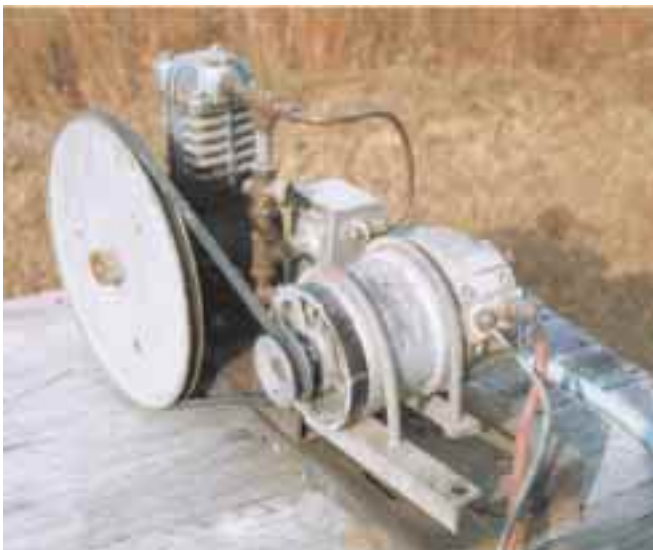
Above: A 24 volt aircraft starter motor run at 12 volts powering this air compressor.
