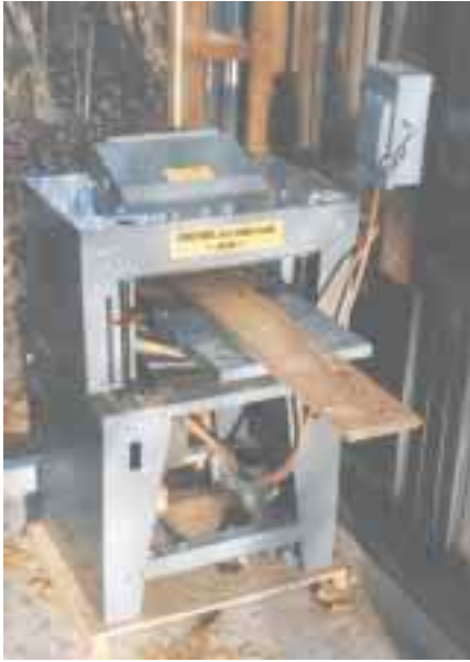
Left: This twelve inch planer is powered by a 24 volt 1 hp DC motor.
