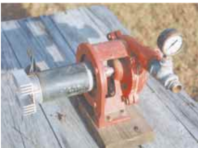
Below: This surplus 12 volt DC motor made a neat conversion for a centrifugal pump.
