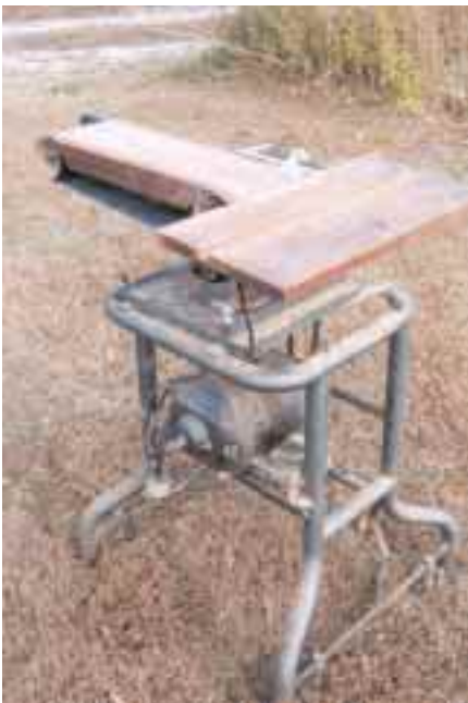
Left: A 12 volt 1/2 hp 1,725 rpm Delco motor found at a flea market powers this belt sander.
