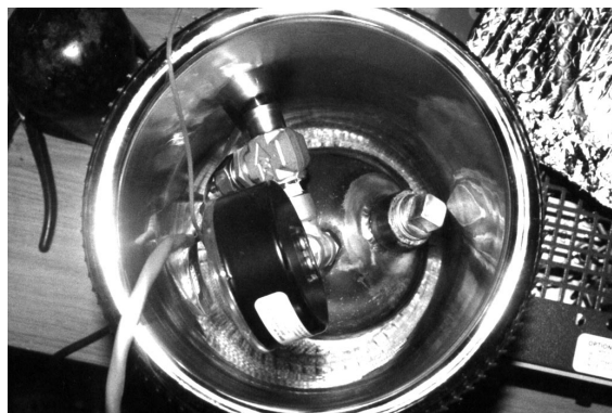
View inside dewar showing Case catalytic fusion cell mounted on resistance heater.
