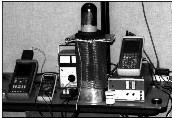
Small Case catalytic fusion cell (inside glass dewar, center) set-up for calorimetry calibration and "live" operation. Note: gas cylinder safety cap is used to secure thermal cover on dewar.
