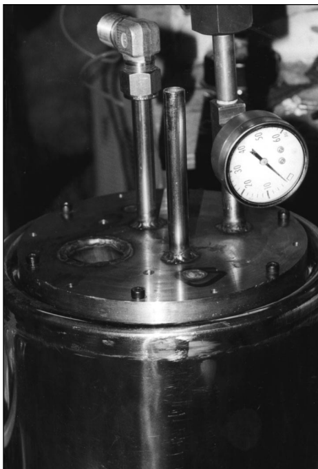
Dr. Case's large modified dewar cell, designed for catalyst beds up to one kilogram and aimed to achieve self-sustaining. Deuterium gas leaks are being fixed.
