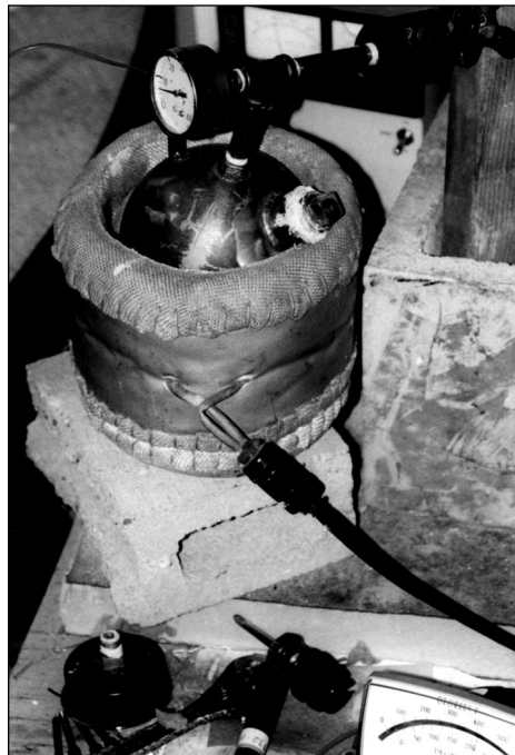
Catalytic fusion reactor in Dr. Les Case's lab, showing pressure gauge and resistance heater collar.
