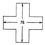
Cut a piece of transparent plastic sheeting (G) to the pattern shown or use five separate pieces of sheeting. Whether using the single or separate sheets, cover the frame with plastic and seal the joints between the sheeting with tape (H). Leave one side of the sheeting loose to be used as a "door" in order to easily remove the plants.
