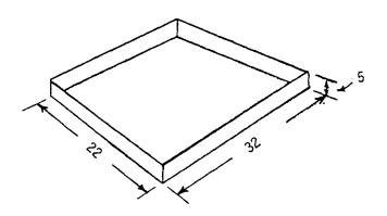
Cut the base from a rectangular tin can (A) to the approximate dimensions given. Adequate bases can also be made from wood, cardboard, sheet metal, etc.
