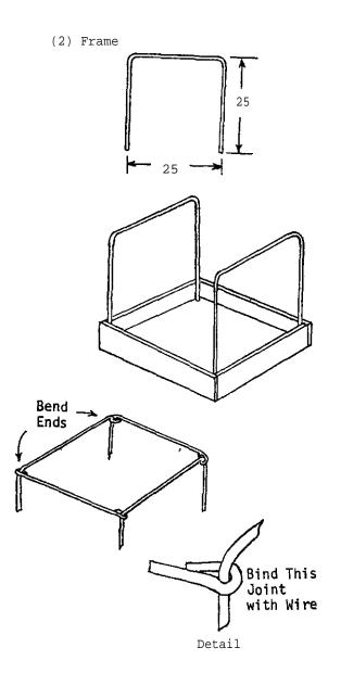
Bend the two longest pieces of soft wire (D) into a "U" shape, and insert the ends into the holes in the base. Fasten the shorter pieces of soft wire (E) to the frame by bending about 1 cm of each end around the bends in the longer wires (D). Bind the joints together with the short, thinner wires (F).
