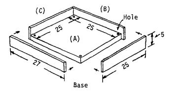
Nail or glue the four rectangular pieces of wood (B,C) to the square piece (A). Drill four holes, 0.2 cm diameter, in the square piece (A), one hole near each corner of the wood.
