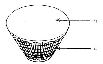
From the wire mesh (K), cut a circle. Cut out and remove the shaded portion as shown. cut a similar but slightly larger shape from the aluminum foil (M). Curve the wire mesh (K) into a cone with an open end that will fit over the base of the incandescent bulb (G), and secure the cut edges together by threading the thin wire (L) in and out of the wire mesh.
