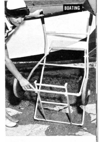
Cart is tilted up to show how single cotter pin (through U bracket) locks platform to bottom rear crosspiece.
