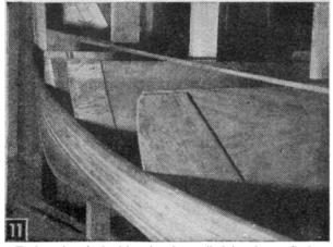
Each strip of planking is edge-nailed in place. Strips flow smoothly around molds.
