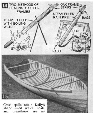
stalled and during planing. face outboard. Put in the inner wales and the seat risers with  $#10 \times 1\frac{1}{2}$  in. fh screws, one in every other frame.
