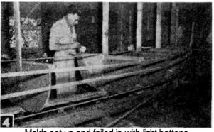
Molds set up and failed in with light battens.
