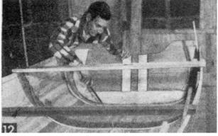
Frame positions are marked out by pencil with thin batten at 5 in. centers. Spring batten from sheer to sheer.
