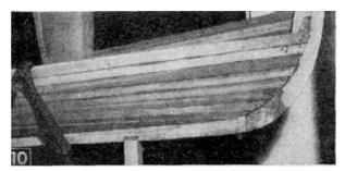
Fort and starboard bottom strip planking applied around forefoot and up the stem.
