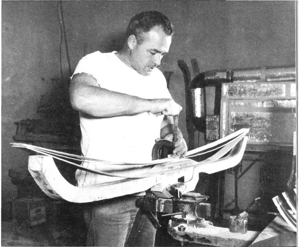
Glue second pair of core laminations, Fibreglas facings to bow assembly and secure to bow form.
