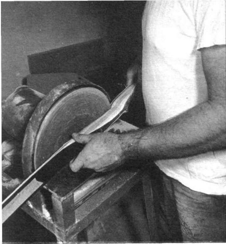
Following the photos on these pages, rough shape the bow handle, on a disc sander if you have one.
