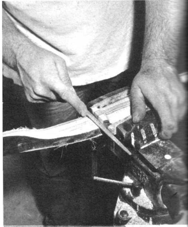
Curve top surface of the arrow rest slightly so that shaft does not rest on too broad a surface.
