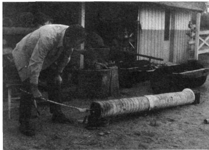
Howard Hill dries his bows with heat of a blow torch directed into improvised drying chamber.
