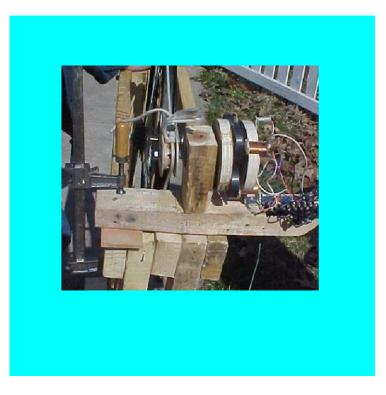
The objective at the time was to demonstrate that "homemade power" could in a post aftermath could be built from salvaged materials available in many areas. The alternator was just a perfect demo to show the main feature, a foot power "WEELIE" that could supply mechanical power for pumps, food grinders, cable linked rotary tool-bits.
