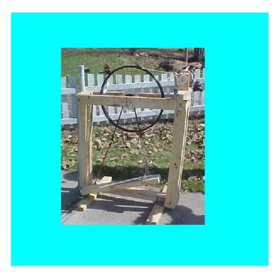
The homemade alternator, built with salvaged microwave magnets and cooling fan coils used LED's to rectify the current, produced about 12 VDC at 1 AMP. This was constructed from a drawing within six days.
