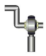
The flywheel hubs are made from 3/8" steel floor flanges sometimes used to support stairway handrails. These were bored out to accept the shaft and the right-hand one cross-drilled through its hub to accept a heavy cotter pin (or high-tech bent nail), tying the wheel securely to the shaft. This arrangement provides adequate stability and has weathered some pretty aggressive use without any problems.
