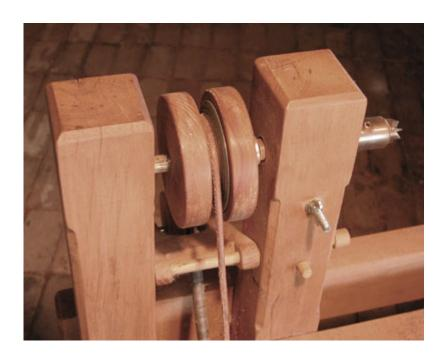
Depending on the type of belt you decide on, you may need a belt-tensioning device of some kind. My belt is made from a couple of Singer treadle sewing machine belts cut and joined to fit the lathe.
