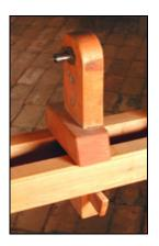
Then again, you could do as I did on my old spring pole lathe. I used a 1/2" x 8" lag screw, with a sharp 90-degree bend in it for a handle. I drilled a 7/16" pilot hole, heated the screw red hot with a propane torch and burn/screwed it into place. With the point reshaped into a smooth, blunt cone and a little paraffin wax rubbed on the threads and point, the "center" worked just fine.
