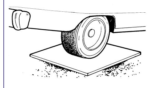
Cover the patch with a piece of scrap plywood or hardboard. Then drive a wheel of a car over the wood and patch. The weight of the car will compact the patch into the hole like a steam roller. Then wait for the patch to harden; brush on the driveway sealer. Let the job set about 36 hours or more before you walk or drive on the freshly-coated surface.
