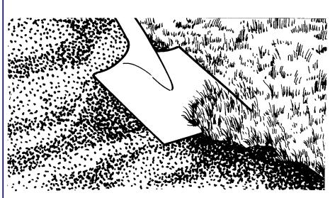
Clean all debris (grass, usually) from the edge of the drive/walkway surface. Then remove all dirt, grease, oil, leaves, twigs, etc., from the surface. You may want to hose down the surface after cleaning. If so, let the surface thoroughly dry before you make patches and apply the surface sealer.
