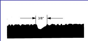
Any crack over 3/8" needs to be filled with patching compound.
