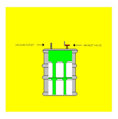
The next picture is a basic hookup between the drum outlet to the engine vacuum line. This hose can be purchased at most auto supply stores, along with a three way connector and a mechanical engine vacuum gauge. Cut hoses to lengths needed, and grease with petroleum jelly the connectors to fit into the hose. My setup also included a small inline gas filter (not shown) to protect the engine in case any dust entered the vacuum line. No hose clamps were needed but one can included them if desired.
