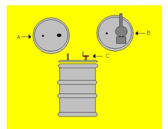
As in (B); if no valve is available, one could attach a homemade "FLAP VALVE" cut out of salvaged auto tire inner tube with its flap hinge end "GOOP 'd" to the lid top.
