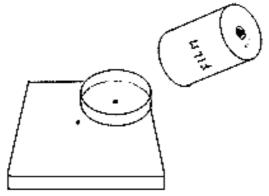
the lid of a 36 mm film box is nailed onto a piece of wood. The wood should be sufficiently heavy to prevent sliding of the eye-holder over the table. The bottom of the box is heated over an alcohol flame and after softening of the plastic one indents the bottom into a concave cup. The centre of the cup is perforated with an awl or a nail.
