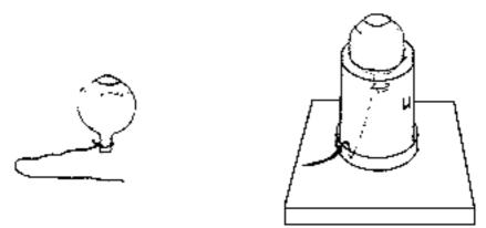
To fixate an eye to this holder one ties a suture around the optic nerve. The suture is then passed through the hole.
