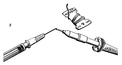
**G**. Trimming the tip of the cryo extractor with a honing stone (or a triangular file/sandpaper and a rough cloth).
