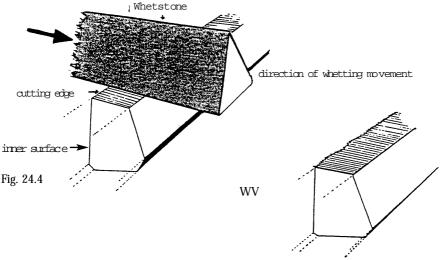
*Note:* Since this surface is very small a bright light can be used. The reflection of the light gives an indication of the angle of the cutting surface. When the light is put in front at eye height the brightest reflexion of the cutting surface will indicate that the cutting surface is horizontal.
