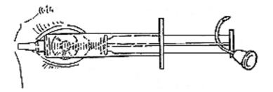
It is essential that the barrel is made of a sufficiently clear plastic to permit viewing of the calibration through the water-filled barrel.
