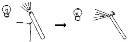
If you give a hard knock with a pen-light on the edge of a table the metal support of the filament in the bulb will deflex. This produces a decentration of the light, sufficiently far of the centre to permit the use of the penlight as a hammerlamp.
