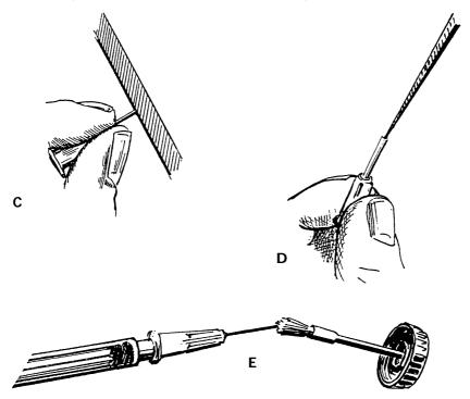
E. Moisten the tip of the needle with a small drop of soldering flux. Do not overfill the canula of the needle with the soldering flux. One should avoid the capillary action. This can be done by closing off the cone of the 16 or 18 G. needle. Put a 1 cc. syringe on the needle, the plunger should be on 0. There should be no air chamber present in the syringe as the flux will tend to reflux inside the needle, which will solder a large part of the lumen.
