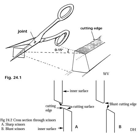
During the sharpening procedure the direction of the sharpening movement has to be checked. If the sharpening direction is from the out side of the scissors towards the inner side, there will be a burr formation on the inner side of the scissor. Before closing the scissors this burr has to be removed, otherwise it will blunt the scissor again. The burr can be removed by scratching it off with your finger nail or with a very fine round whetstone removing it with a turning movement.
